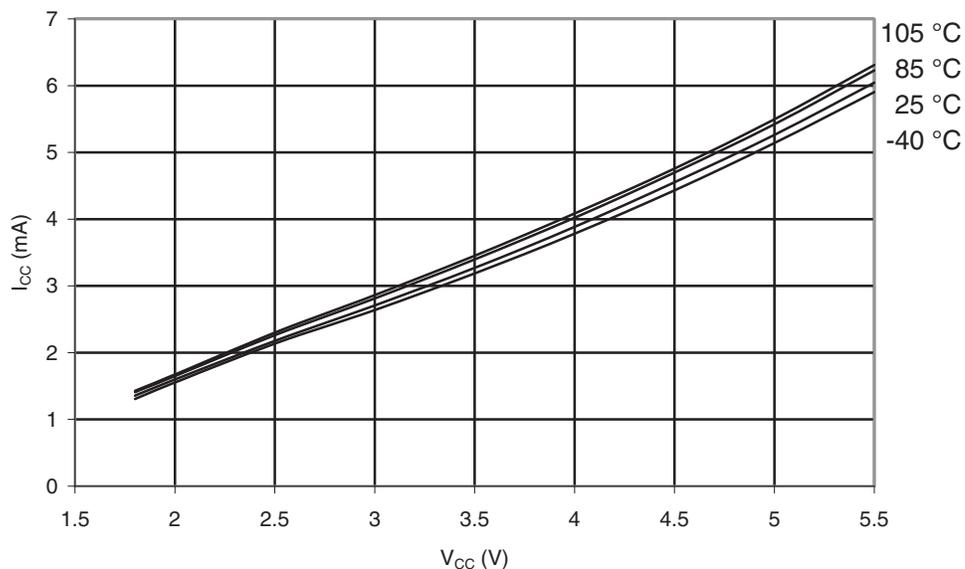
**Figure 31-82. Active Supply Current vs. V<sub>CC</sub> (Internal RC Oscillator, 1 MHz)**
