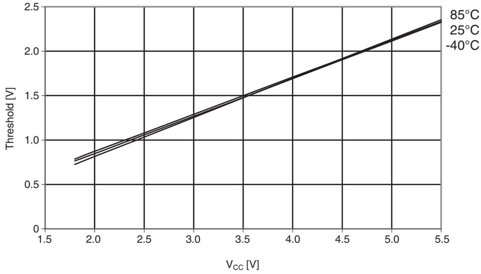
**Figure 30-79. ATmega164PA: Reset pin input hysteresis vs.  $V_{CC}$**
