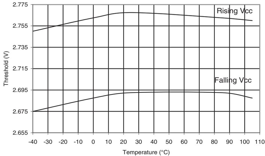
**Figure 31-107. BOD Threshold vs. Temperature ( $V_{CC} = 1.8V$ )**
