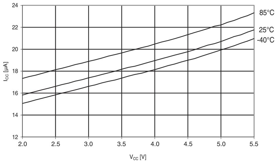
**Figure 30-241. ATmega644A: Programming current vs.  $V_{CC}$**
