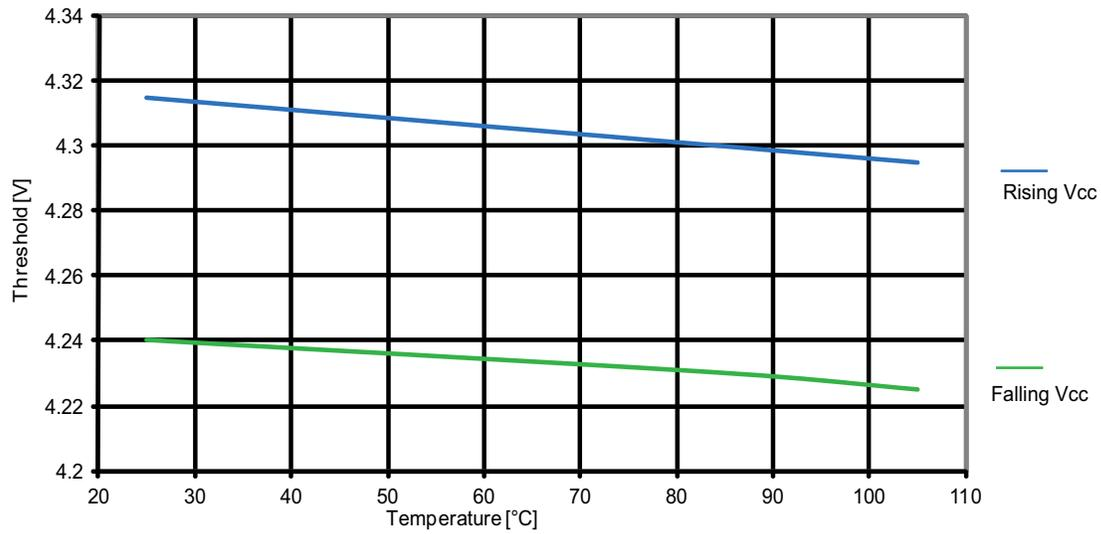
**Figure 31-26. ATmega164PA: BOD threshold vs. temperature ( $V_{BOT} = 2.7V$ )**
