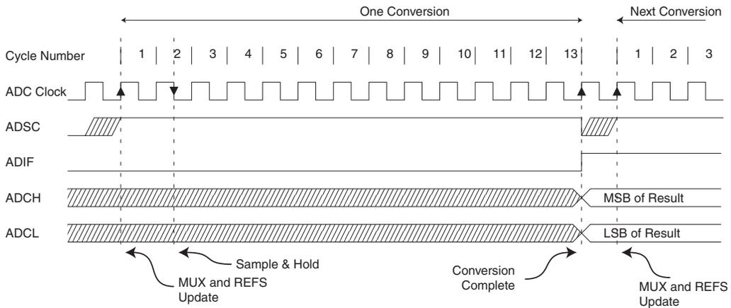
**Figure 23-6. ADC Timing diagram, auto triggered conversion**
