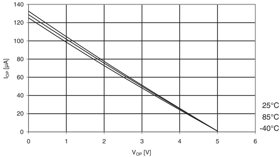
**Figure 30-67. ATmega164PA: Reset pull-up resistor current vs. reset pin voltage ( $V_{CC} = 1.8V$ )**
