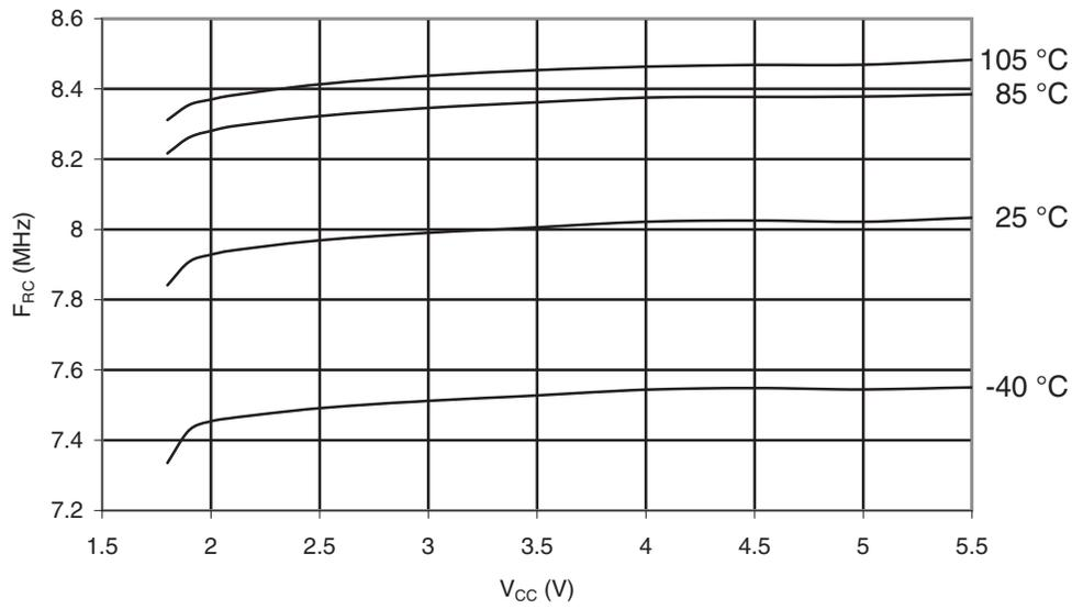
**Figure 31-72. Calibrated 8 MHz RC Oscillator vs. Temperature**
