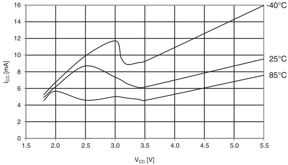
**Figure 30-242. ATmega644A: Watchdog timer current vs.  $V_{CC}$**
