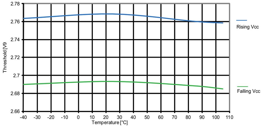
**Figure 31-27. ATmega164PA: BOD threshold vs. temperature ( $V_{BOT} = 1.8V$ )**
