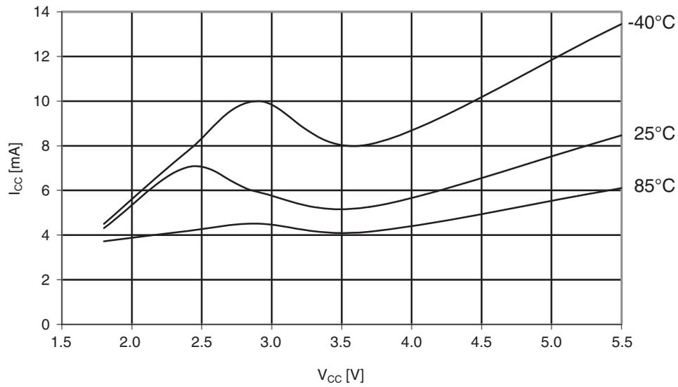
**Figure 30-341. ATmega1284: Watchdog timer current vs.  $V_{CC}$**
