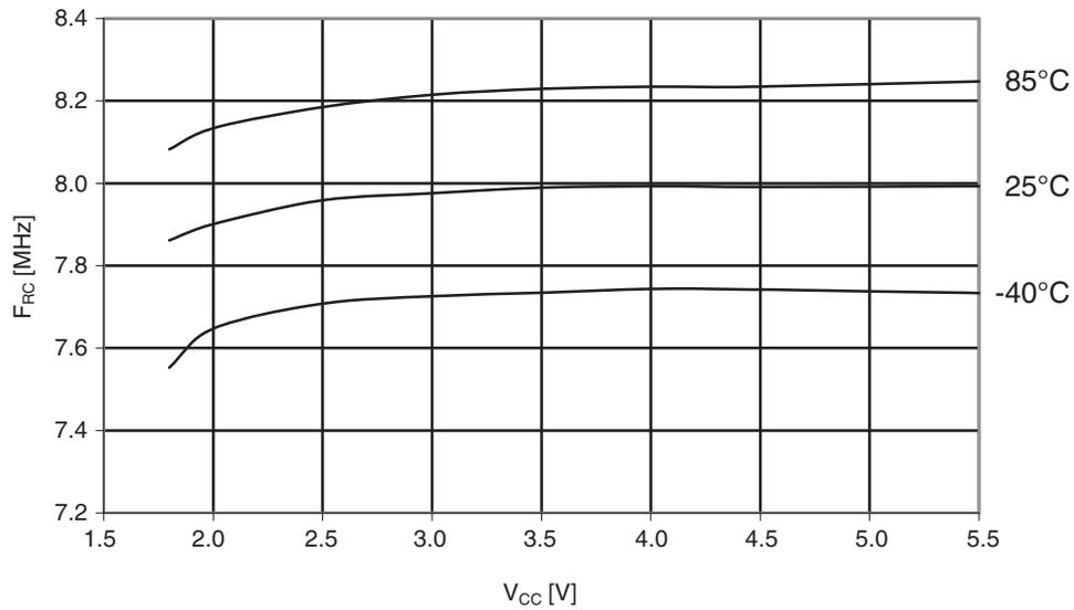
**Figure 30-39. ATmega164A: Calibrated 8MHz RC oscillator vs. temperature**
