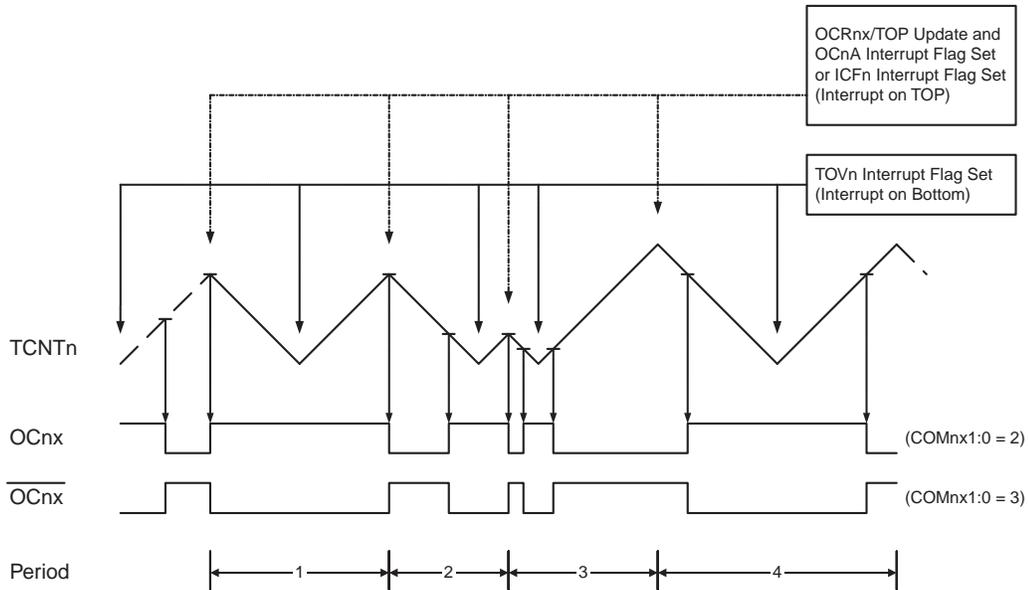
The Timer/Counter Overflow Flag (TOVn) is set each time the counter reaches BOTTOM. When either OCRnA or ICRn is used for defining the TOP value, the OCnA or ICFn Flag is set accordingly at the same timer clock cycle as the OCRnx Registers are updated with the double buffer value (at TOP). The Interrupt Flags can be used to generate an interrupt each time the counter reaches the TOP or BOTTOM value.
