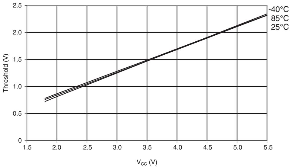
**Figure 30-325. ATmega1284: Reset pin input hysteresis vs.  $V_{CC}$**
