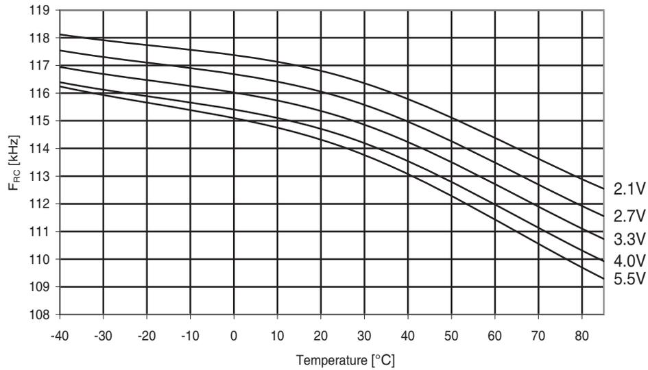
**Figure 30-233. ATmega644A: Watchdog oscillator frequency vs.  $V_{CC}$**
