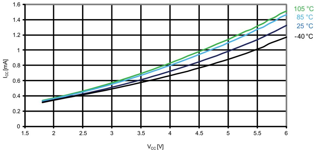
**Figure 31-124. ATmega1284P: Idle supply current vs.  $V_{CC}$  (internal RC oscillator, 1MHz)**
