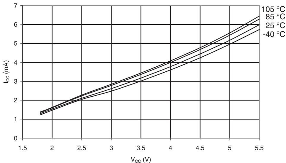
**Figure 31-43. Active Supply Current vs.  $V_{CC}$  (Internal RC Oscillator, 1 MHz)**
