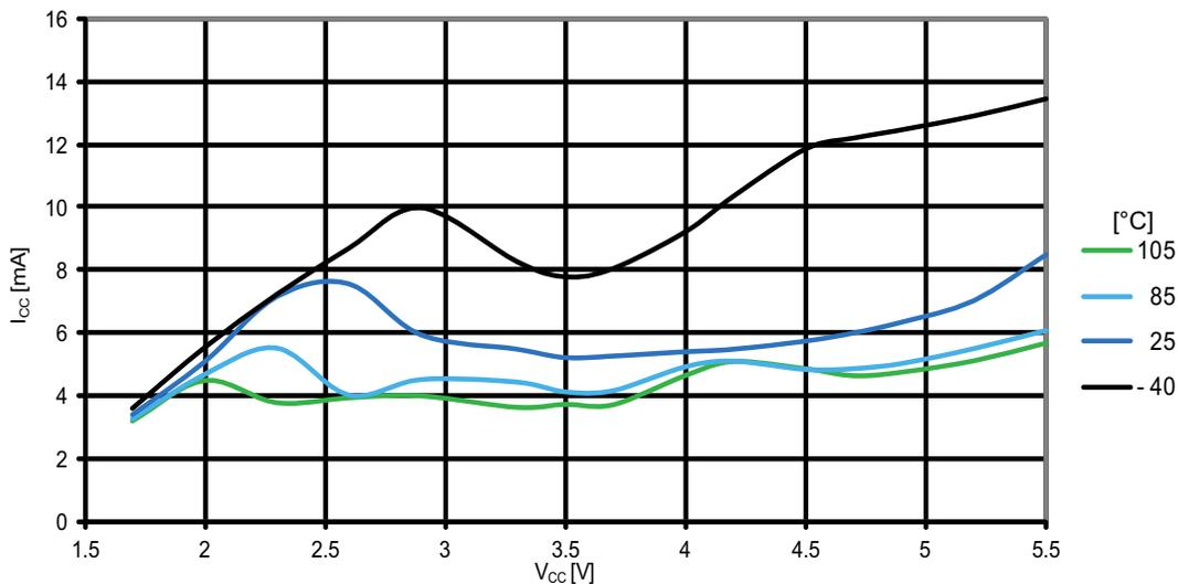
**Figure 31-161. ATmega1284P: Watchdog timer current vs.  $V_{CC}$**
