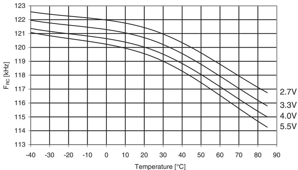
**Figure 30-382. ATmega1284P: Watchdog oscillator frequency vs.  $V_{CC}$**
