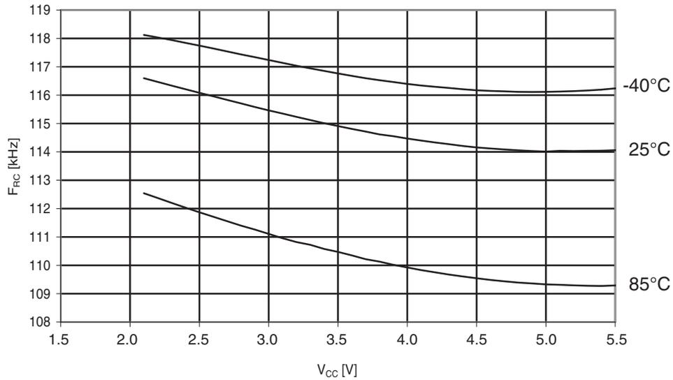
**Figure 30-234. ATmega644A: Calibrated 8MHz RC oscillator vs.  $V_{CC}$**
