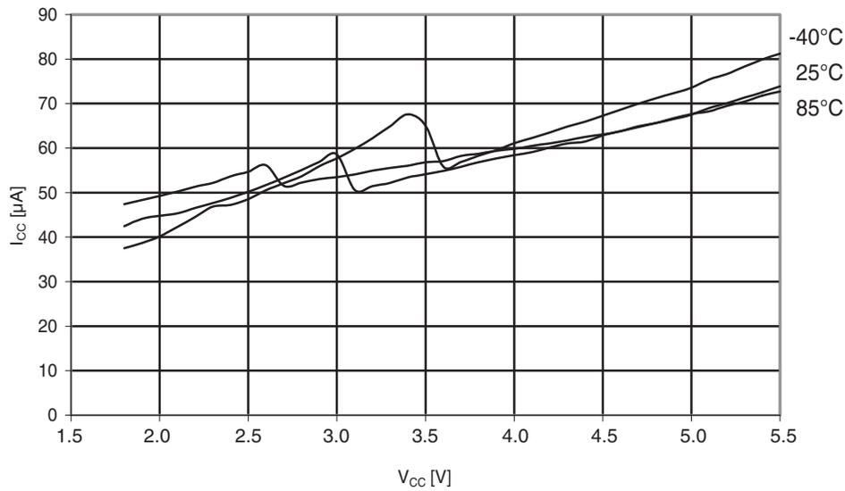
Figure 30-141. ATmega324A: AREF external reference current vs.  $V_{CC}$
