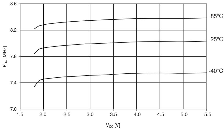
Figure 30-186. ATmega324PA: Calibrated 8MHz RC oscillator vs. temperature
