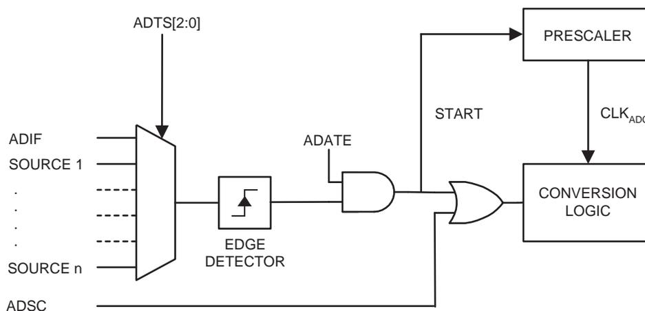
Using the ADC Interrupt Flag as a trigger source makes the ADC start a new conversion as soon as the ongoing conversion has finished. The ADC then operates in Free Running mode, constantly sampling and updating the ADC Data Register. The first conversion must be started by writing a logical one to the ADSC bit in ADCSRA. In
