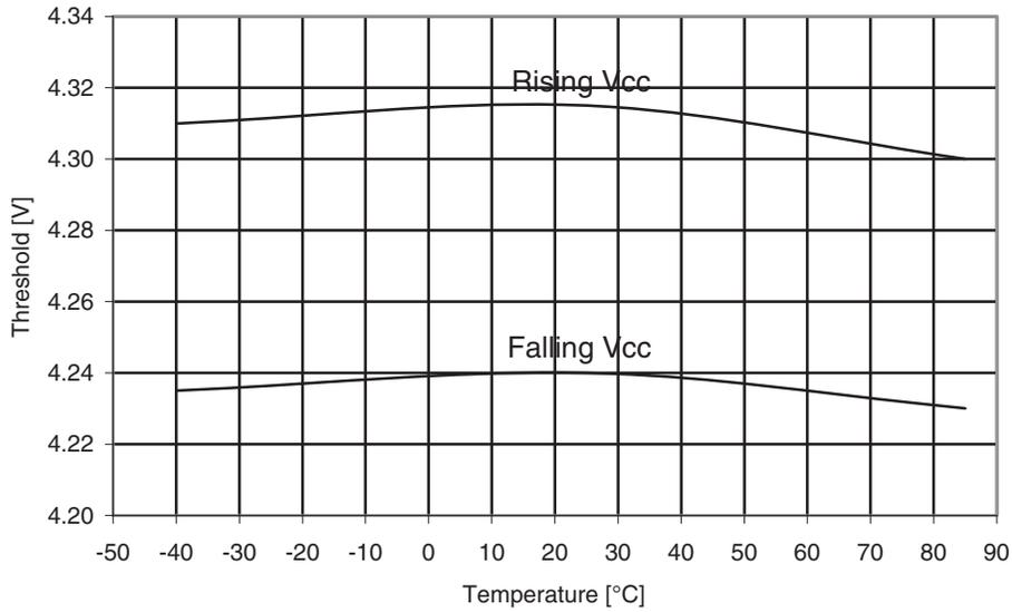
**Figure 30-32. ATmega164A: BOD threshold vs. temperature ( $V_{BOT} = 2.7V$ )**
