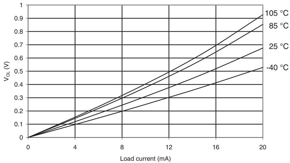
Figure 31-57. I/O Pin Output Voltage vs. Sink Current ( $V_{CC} = 5V$ )
