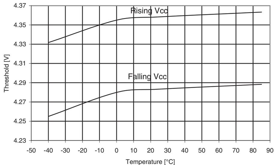
Figure 30-377. ATmega1284P: BOD threshold vs. temperature ( $V_{BOT} = 2.7V$ )
