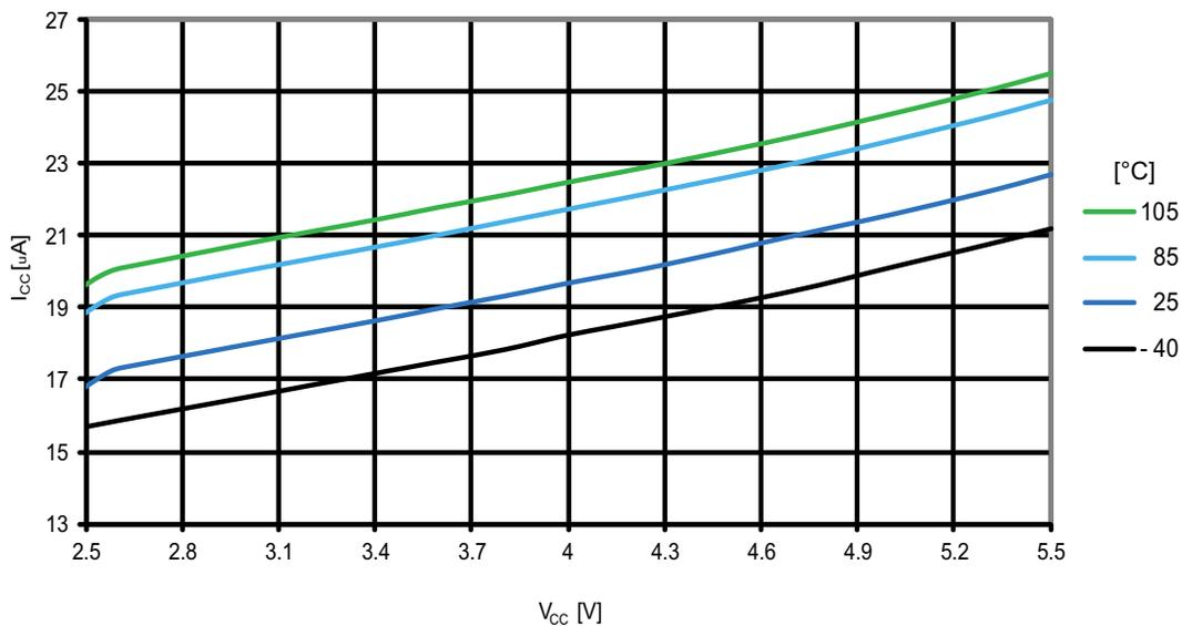
**Figure 31-160. ATmega1284P: Programming current vs.  $V_{CC}$**
