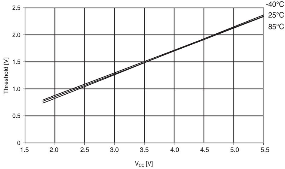
**Figure 30-177. ATmega324PA: Reset pin input hysteresis vs.  $V_{CC}$**
