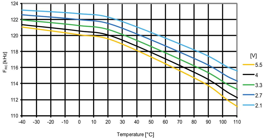
Figure 31-152. ATmega1284P: Watchdog oscillator frequency vs. V<sub>CC</sub>
