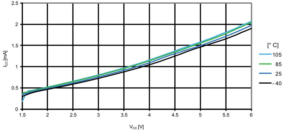
**Figure 31-122. ATmega1284P: Active supply current vs.  $V_{CC}$  (internal RC oscillator, 128kHz)**
