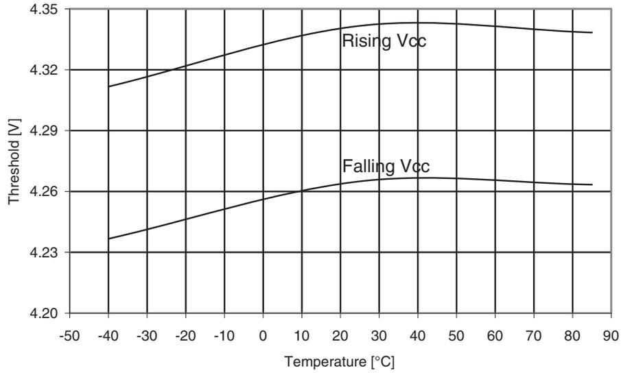
**Figure 30-228. ATmega644A: BOD threshold vs. temperature ( $V_{BOT} = 2.7V$ )**
