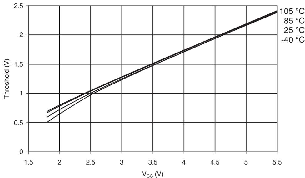
**Figure 31-101. I/O Pin Input Hysteresis vs.  $V_{CC}$**
