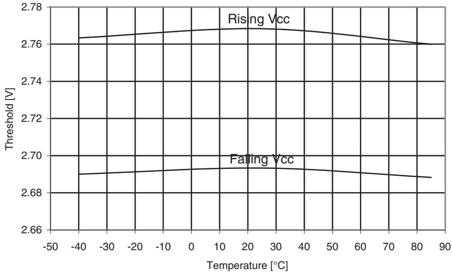
**Figure 30-33. ATmega164A: BOD threshold vs. temperature ( $V_{BOT} = 1.8V$ )**
