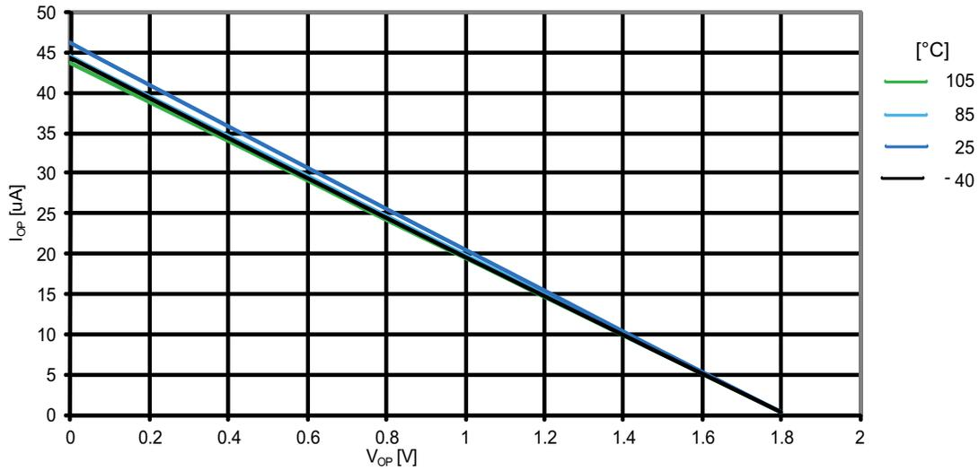
**Figure 31-10. ATmega164PA: I/O pin pull-up resistor current vs. input voltage ( $V_{CC} = 2.7V$ )**
