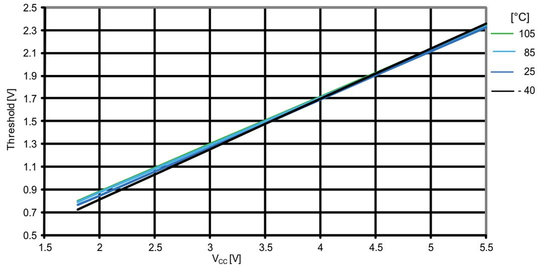
**Figure 31-24. ATmega164PA: Reset pin input hysteresis vs.  $V_{CC}$**
