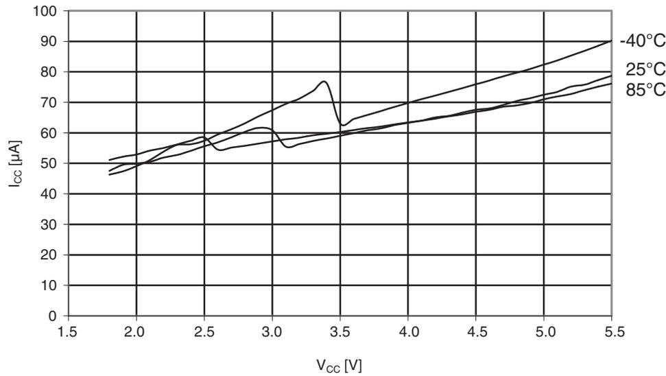
**Figure 30-43. ATmega164A: AREF external reference current vs.  $V_{CC}$**
