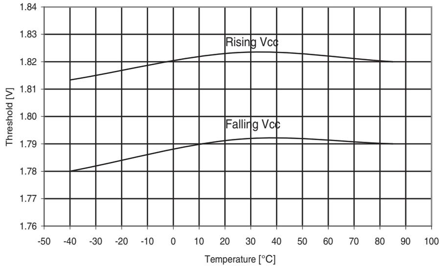
**Figure 30-279. ATmega644PA: Calibrated bandgap voltage vs.  $V_{CC}$**
