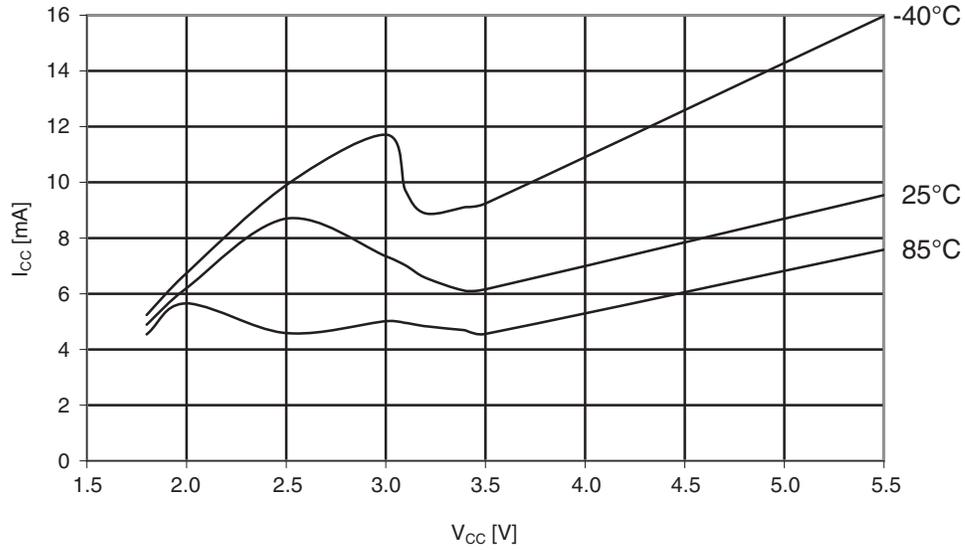
**Figure 30-291. ATmega644PA: Watchdog timer current vs.  $V_{CC}$**
