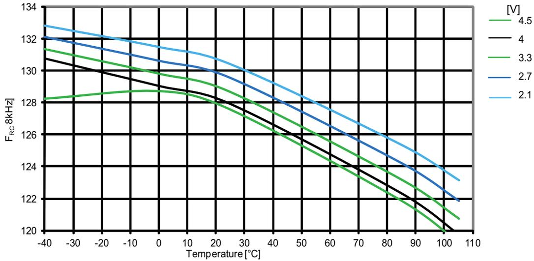
**Figure 31-31. ATmega164PA: Watchdog oscillator frequency vs.  $V_{CC}$**
