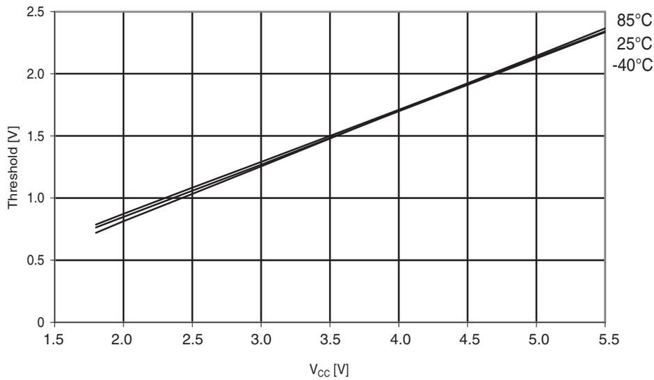
**Figure 30-223. ATmega644A: I/O pin input hysteresis vs.  $V_{CC}$**
