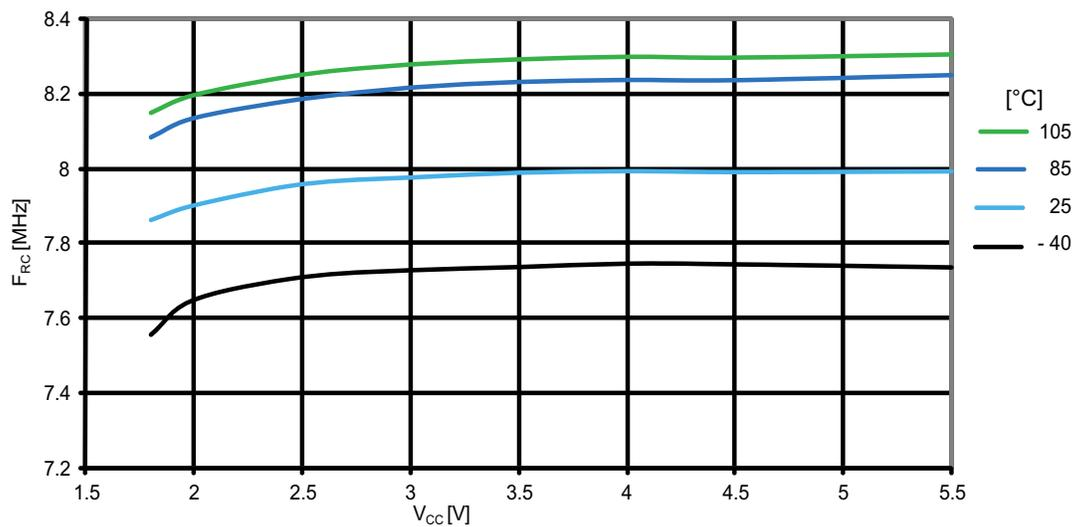
**Figure 31-33. ATmega164PA: Calibrated 8MHz RC oscillator vs. temperature**
