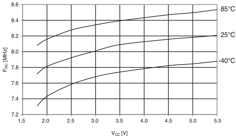
**Figure 30-384. ATmega1284P: Calibrated 8MHz RC oscillator vs. temperature**
