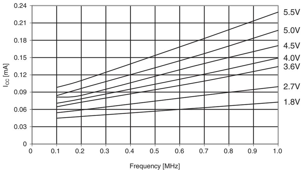
**Figure 30-301. ATmega1284: Idle supply current vs. frequency (1 - 20MHz)**
