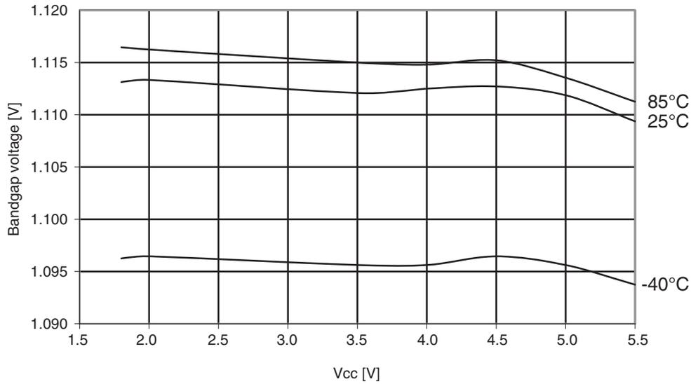
**Figure 30-380. ATmega1284P: Bandgap voltage vs. temperature**
