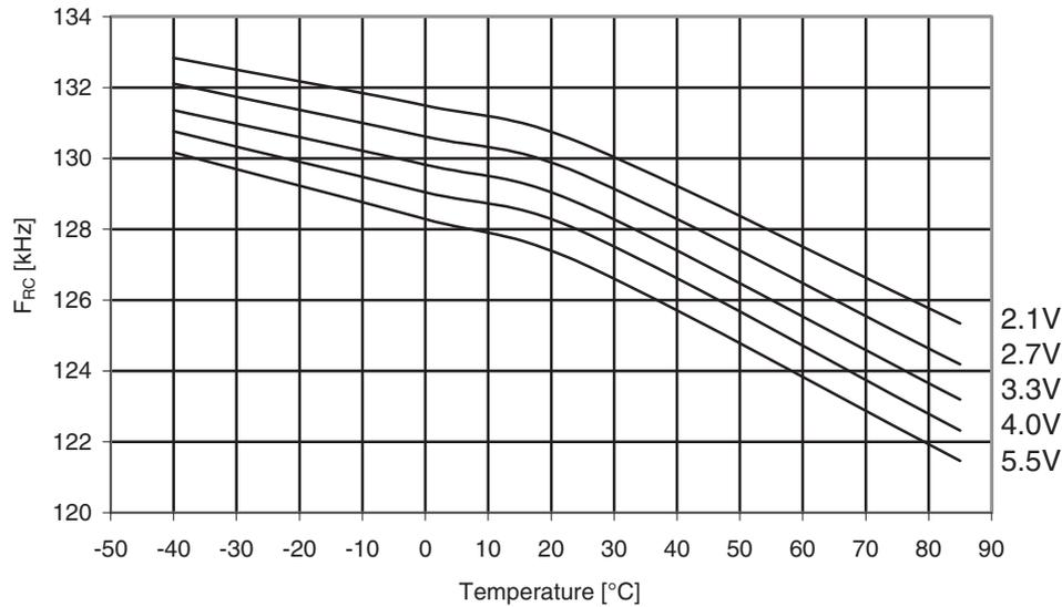
**Figure 30-37. ATmega164A: Watchdog oscillator frequency vs.  $V_{CC}$**
