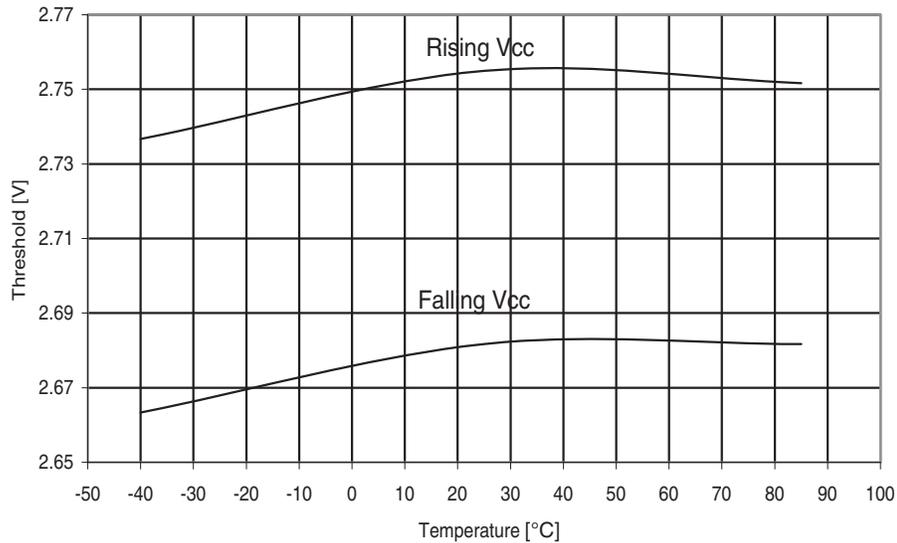
**Figure 30-278. ATmega644PA: BOD threshold vs. temperature ( $V_{BOT} = 1.8V$ )**
