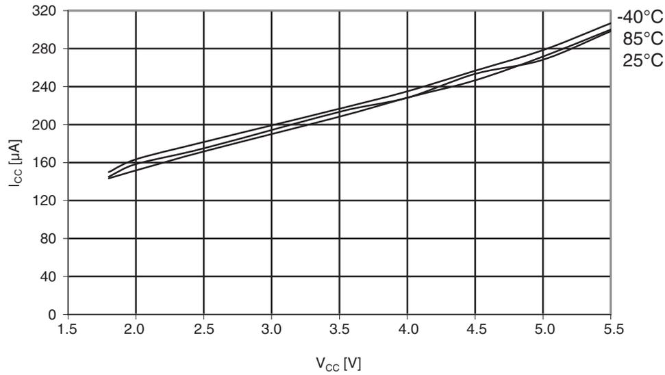
**Figure 30-42. ATmega164A: Analog comparator current vs.  $V_{CC}$**
