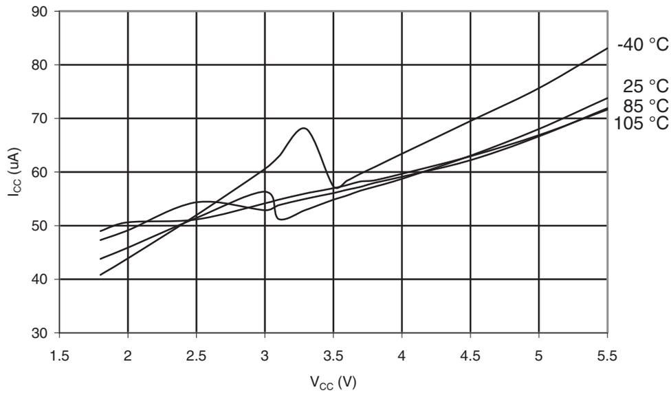
**Figure 31-115. AREF External Reference Current vs.  $V_{CC}$**
