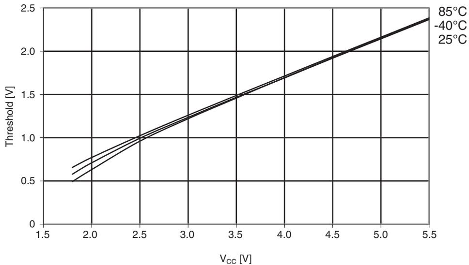
**Figure 30-372. ATmega1284P: I/O pin input hysteresis vs.  $V_{CC}$**
