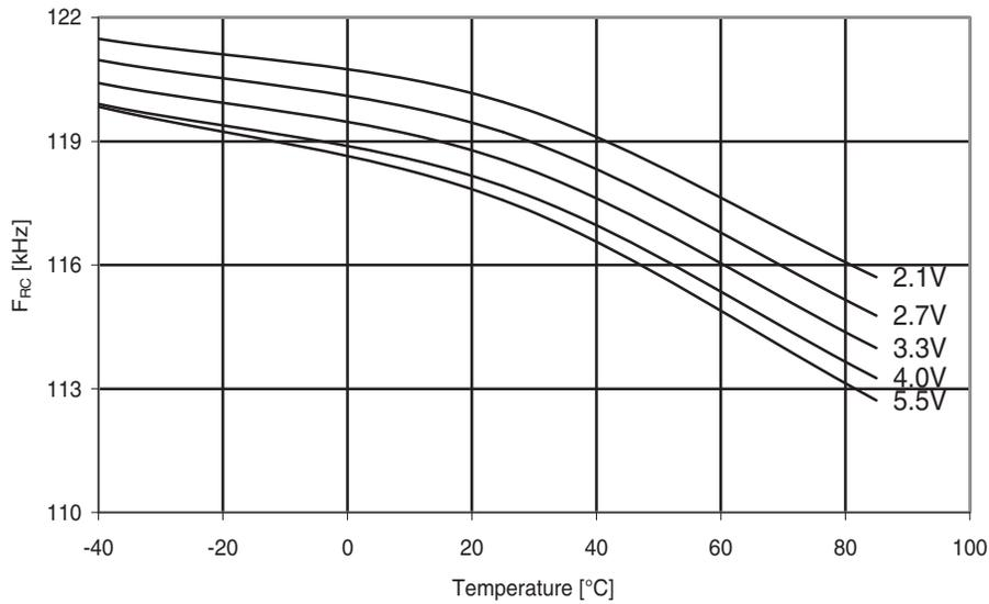
**Figure 30-135. ATmega324A: Watchdog oscillator frequency vs.  $V_{CC}$**
