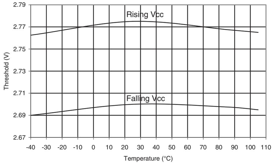
**Figure 31-68. BOD Threshold vs. Temperature ( $V_{CC} = 1.8V$ )**
