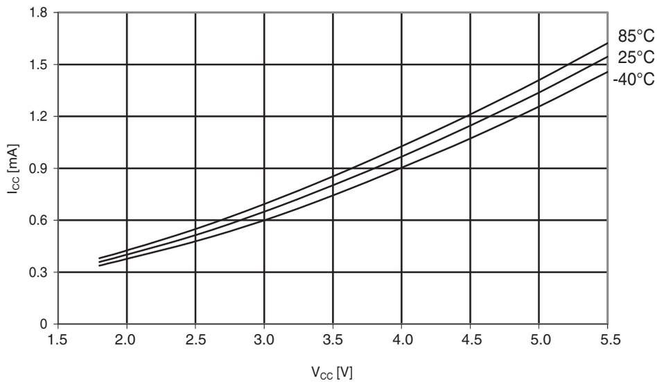
**Figure 30-107. ATmega324A: Idle supply current vs.  $V_{CC}$  (internal RC oscillator, 1MHz)**
