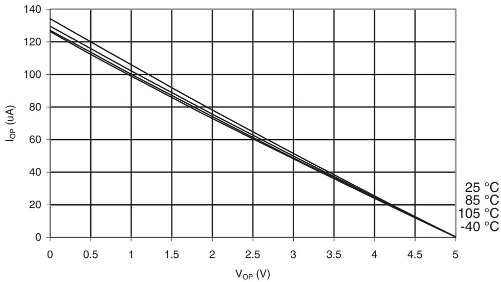
**Figure 31-53. Reset Pull-up Resistor Current vs. Reset Pin Voltage ( $V_{CC} = 1.8V$ )**
