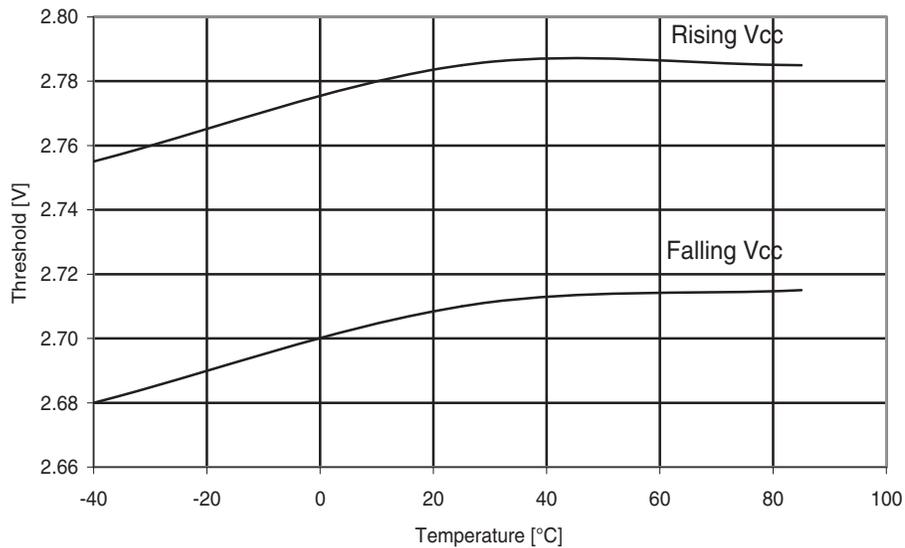
**Figure 30-180. ATmega324PA: BOD threshold vs. temperature ( $V_{BOT} = 1.8V$ )**
