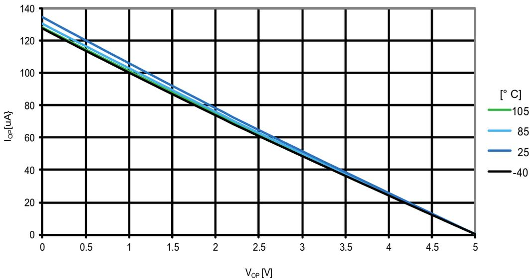
**Figure 31-132. ATmega1284P: Reset pull-up resistor current vs. reset pin voltage ( $V_{CC} = 1.8V$ )**
