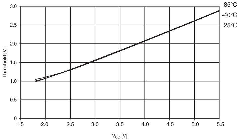
**Figure 30-173. ATmega324PA: I/O pin input threshold vs.  $V_{CC}$  ( $V_{IL}$ , I/O pin read as '0')**
