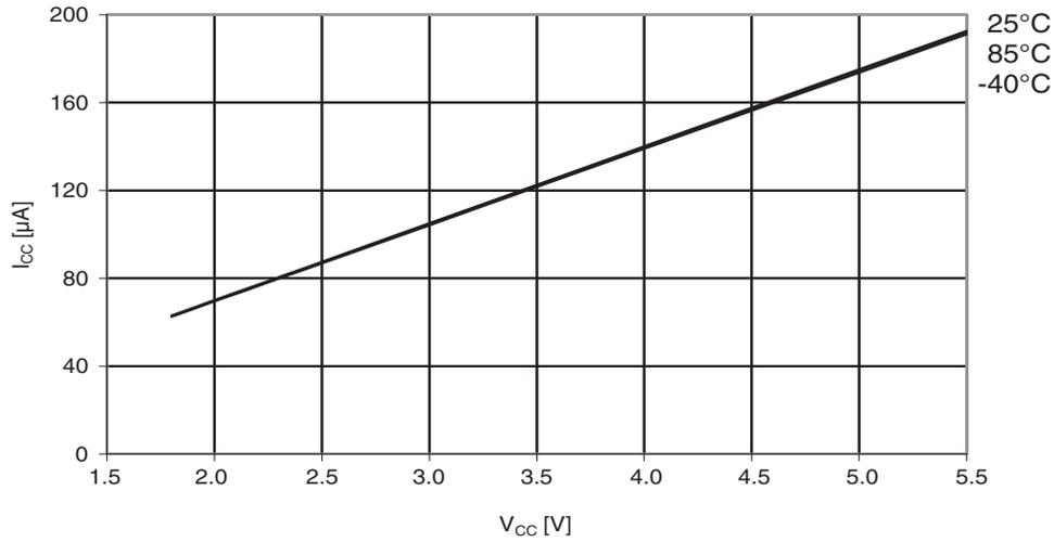
**Figure 30-44. ATmega164A: Brownout detector current vs.  $V_{CC}$**
