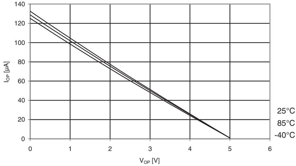
**Figure 30-18. ATmega164A: Reset pull-up resistor current vs. reset pin voltage ( $V_{CC} = 1.8V$ )**
