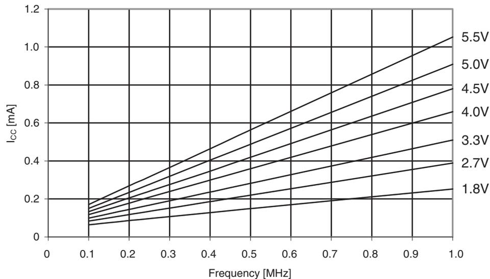
Figure 30-51. ATmega164PA: Active supply current vs. frequency (1 - 20MHz)
