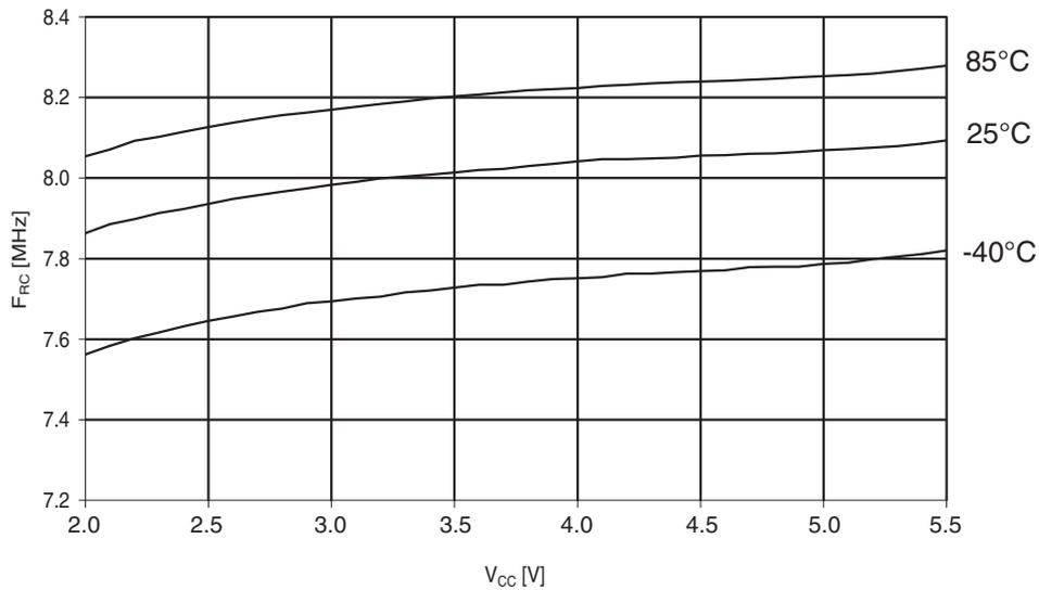
**Figure 30-235. ATmega644A: Calibrated 8MHz RC oscillator vs. temperature**
