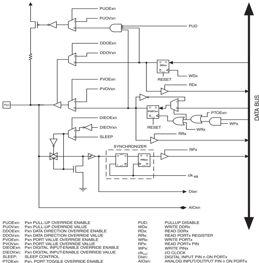
Note: 1. WRx, WPx, WDx, RRx, RPx, and RDx are common to all pins within the same port. clk<sub>I/O</sub>, SLEEP, and PUD are common to all ports. All other signals are unique for each pin.
