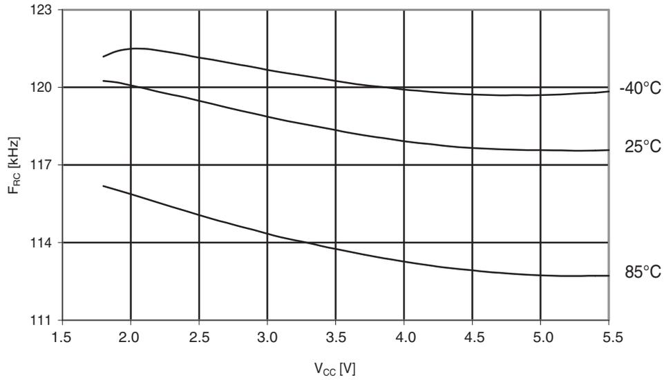
**Figure 30-136. ATmega324A: Calibrated 8MHz RC oscillator vs.  $V_{CC}$**
