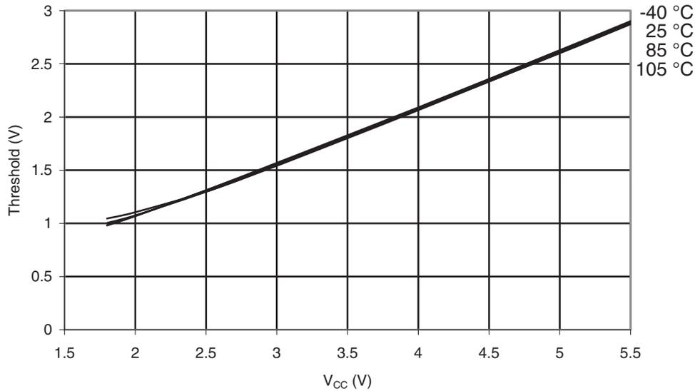
**Figure 31-61. I/O Pin Input Threshold vs.  $V_{CC}$  ( $V_{IL}$ , I/O Pin Read as '0')**
