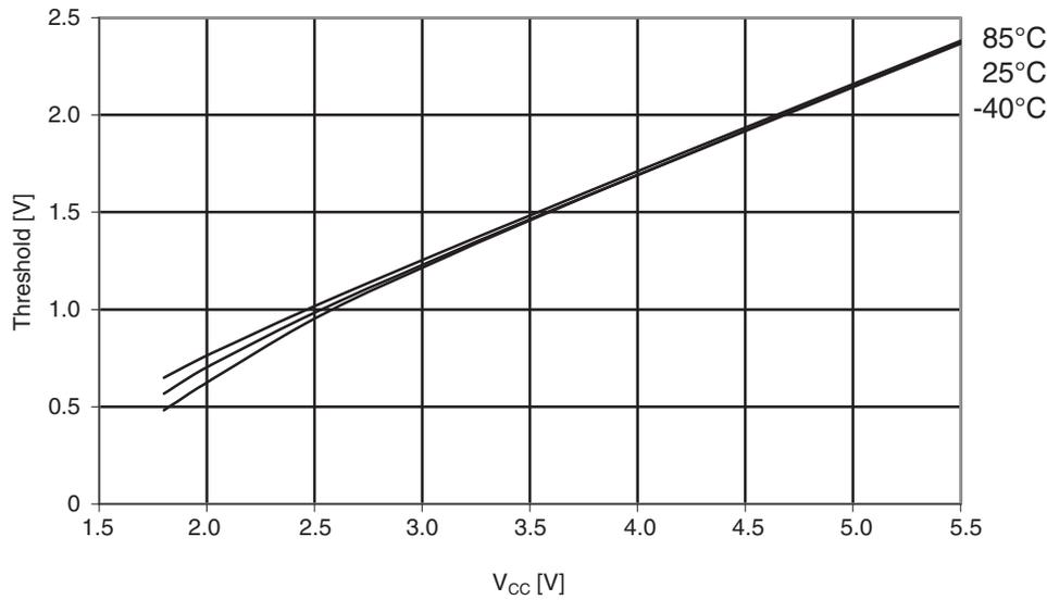
**Figure 30-76. ATmega164PA: I/O pin input hysteresis vs.  $V_{CC}$**
