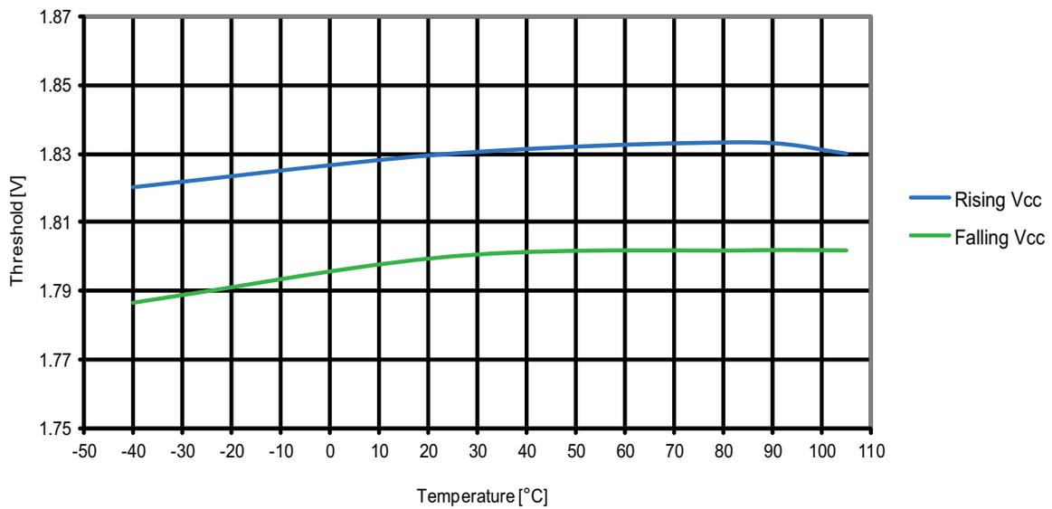
**Figure 31-149. ATmega1284P: Calibrated bandgap voltage vs.  $V_{CC}$**
