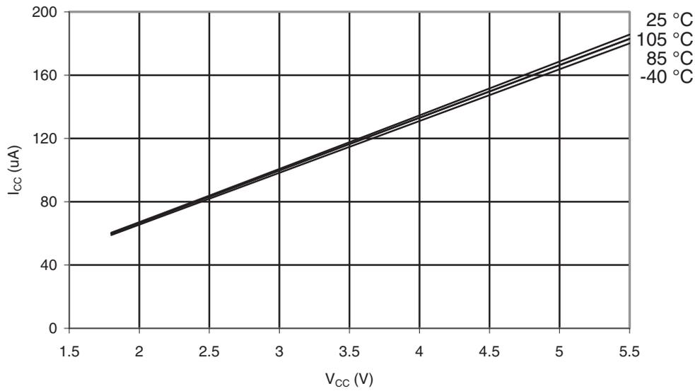
**Figure 31-77. Brownout Detector Current vs.  $V_{CC}$**
