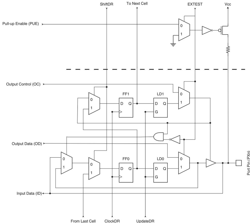
**Figure 25-4. General Port Pin schematic diagram**
