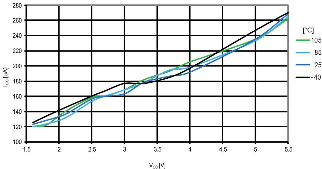
**Figure 31-157. ATmega1284P: Analog comparator current vs.  $V_{CC}$**
