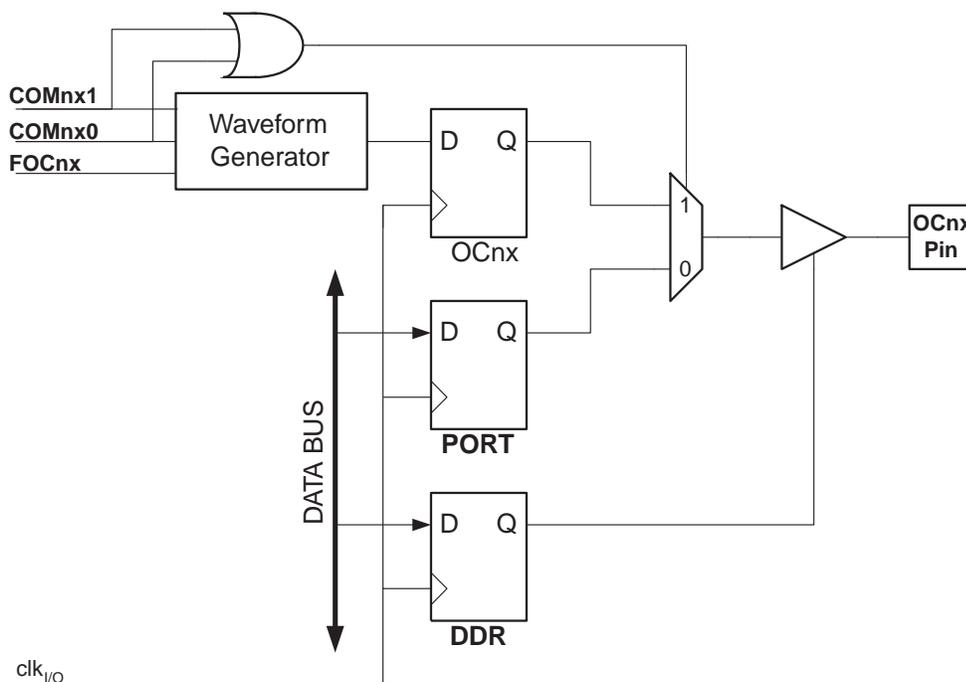
The general I/O port function is overridden by the Output Compare (OC2x) from the Waveform Generator if either of the COM2x1:0 bits are set. However, the OC2x pin direction (input or output) is still controlled by the Data Direction Register (DDR) for the port pin. The Data Direction Register bit for the OC2x pin (DDR\_OC2x) must be set as output before the OC2x value is visible on the pin. The port override function is independent of the Waveform Generation mode.
