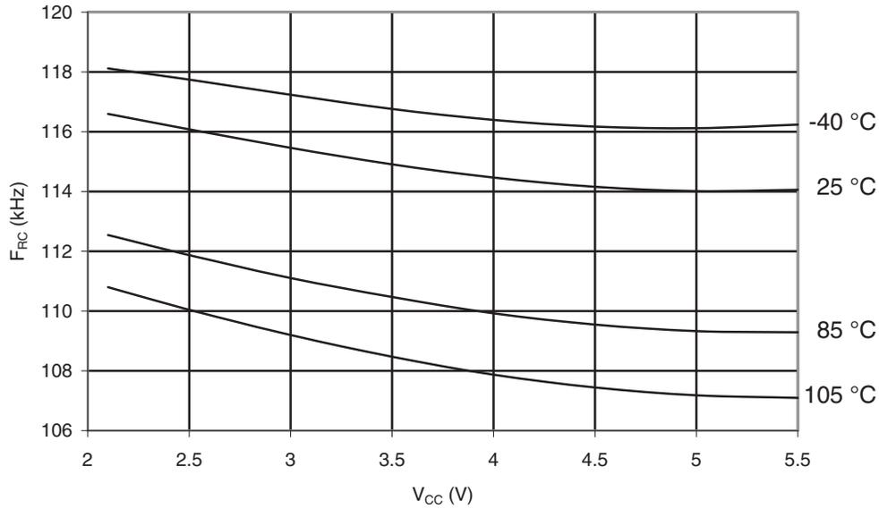
**Figure 31-110. Calibrated 8 MHz RC Oscillator vs.  $V_{CC}$**
