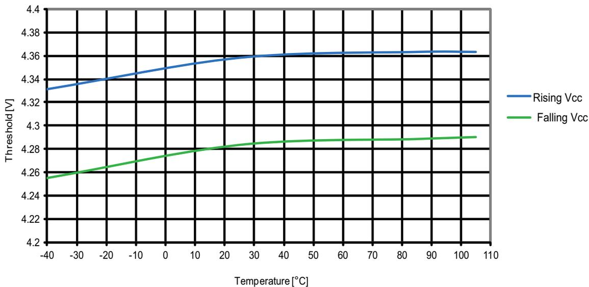
**Figure 31-147. ATmega1284P: BOD threshold vs. temperature ( $V_{BOT} = 2.7V$ )**
