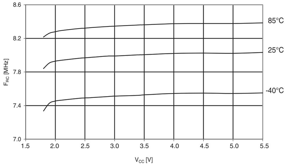
**Figure 30-137. ATmega324A: Calibrated 8MHz RC oscillator vs. temperature**
