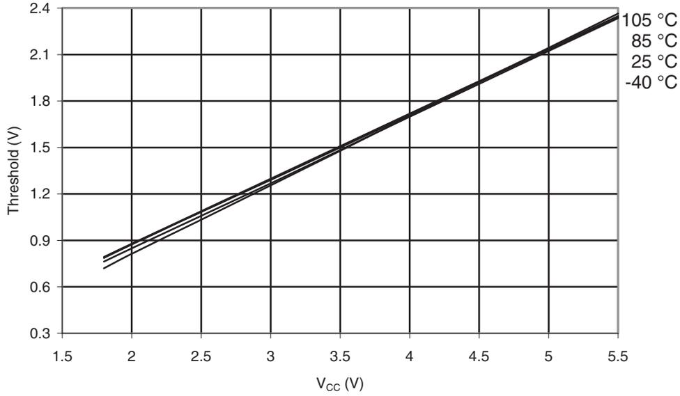
**Figure 31-104. Reset Pin Input Hysteresis vs.  $V_{CC}$**
