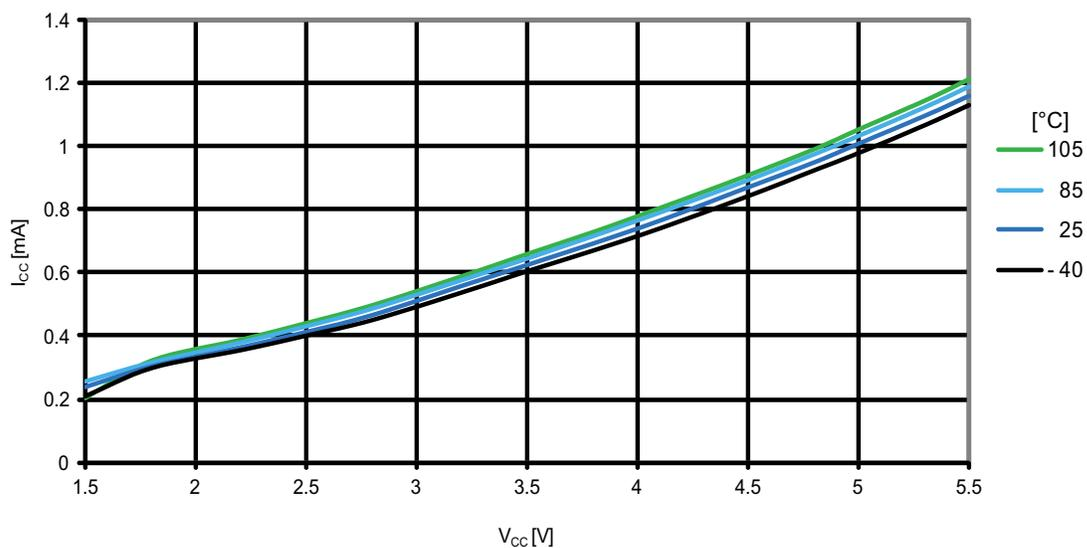
**Figure 31-3. ATmega164PA: Active supply current vs.  $V_{CC}$  (internal RC oscillator, 128kHz)**
