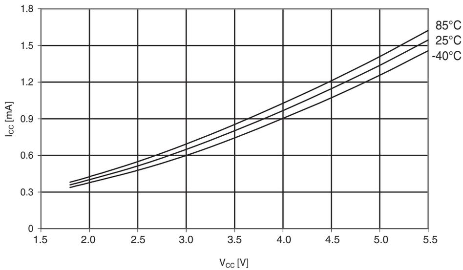
**Figure 30-156. ATmega324PA: Idle supply current vs.  $V_{CC}$  (internal RC oscillator, 1MHz)**
