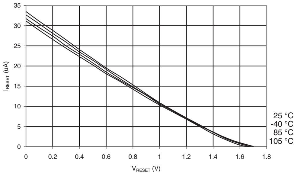
**Figure 31-93. Reset Pull-up Resistor Current vs. Reset Pin Voltage ( $V_{CC} = 2.7V$ )**
