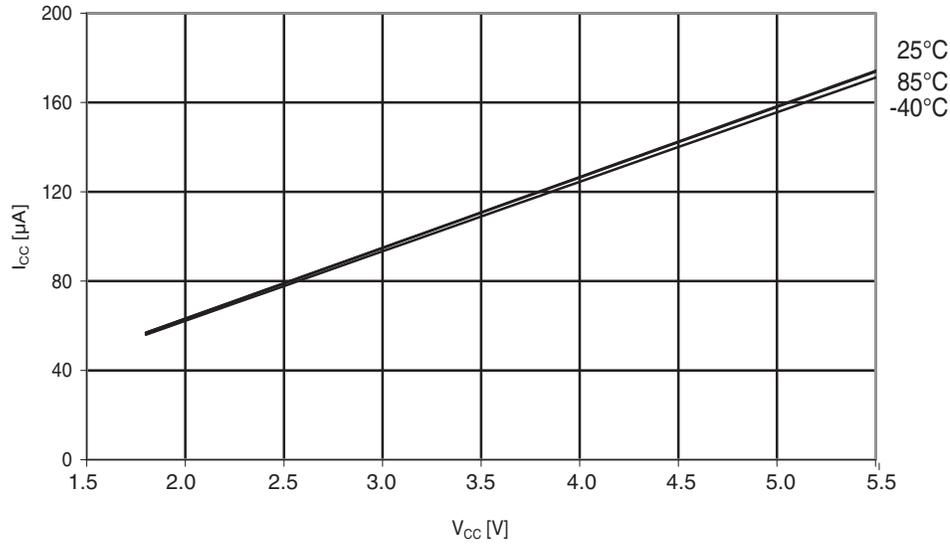
Figure 30-289. ATmega644PA: Brownout detector current vs.  $V_{CC}$
