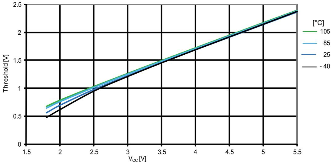
**Figure 31-21. ATmega164PA: I/O pin input hysteresis vs.  $V_{CC}$**
