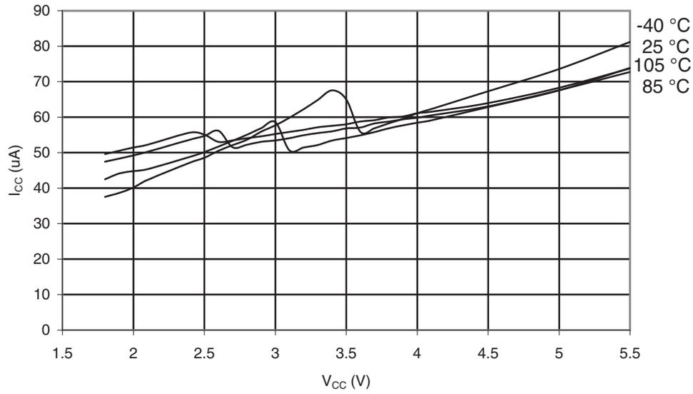
**Figure 31-76. AREF External Reference Current vs.  $V_{CC}$**
