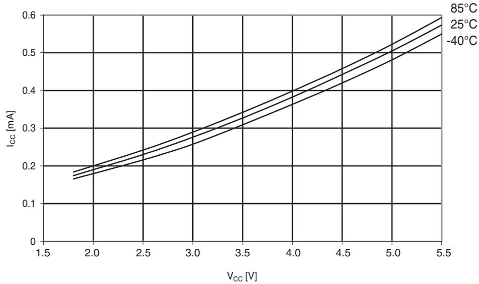
**Figure 30-108. ATmega324A: Idle supply current vs.  $V_{CC}$  (internal RC oscillator, 128kHz)**
