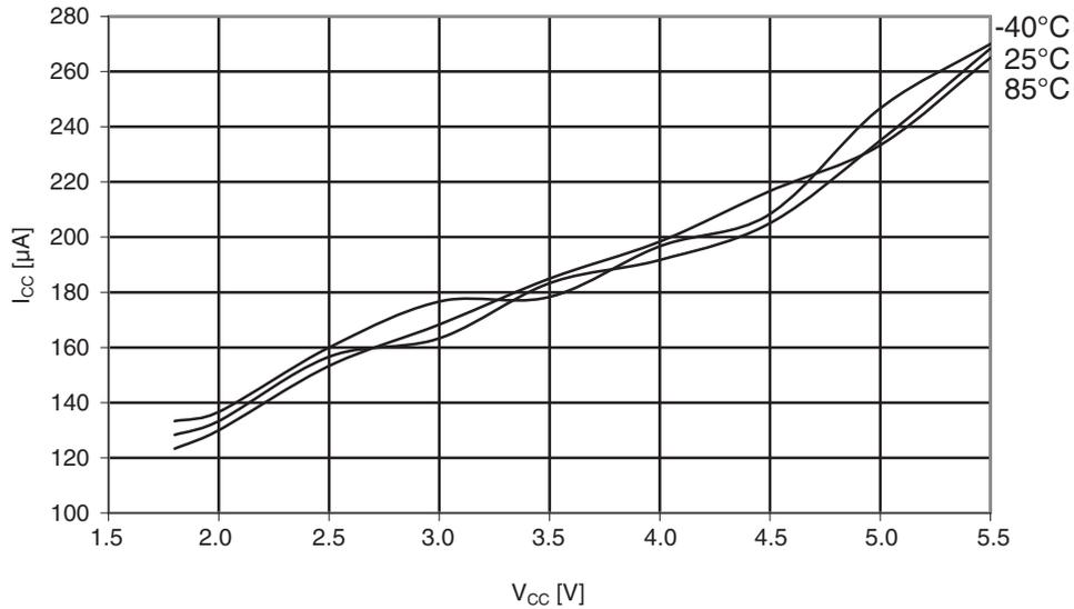
Figure 30-387. ATmega1284P: Analog comparator current vs.  $V_{CC}$
