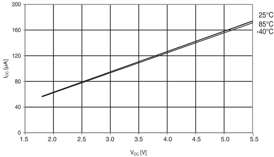
Figure 30-240. ATmega644A: Brownout detector current vs.  $V_{CC}$
