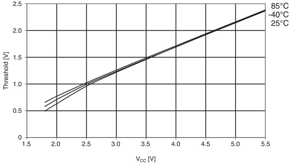
**Figure 30-322. ATmega1284: I/O pin input hysteresis vs.  $V_{CC}$**
