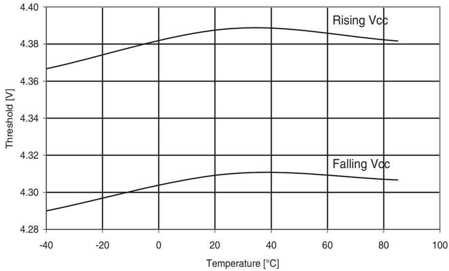
**Figure 30-130. ATmega324A: BOD threshold vs. temperature ( $V_{BOT} = 2.7V$ )**
