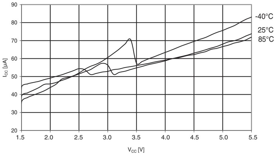
Figure 30-239. ATmega644A: AREF external reference current vs.  $V_{CC}$
