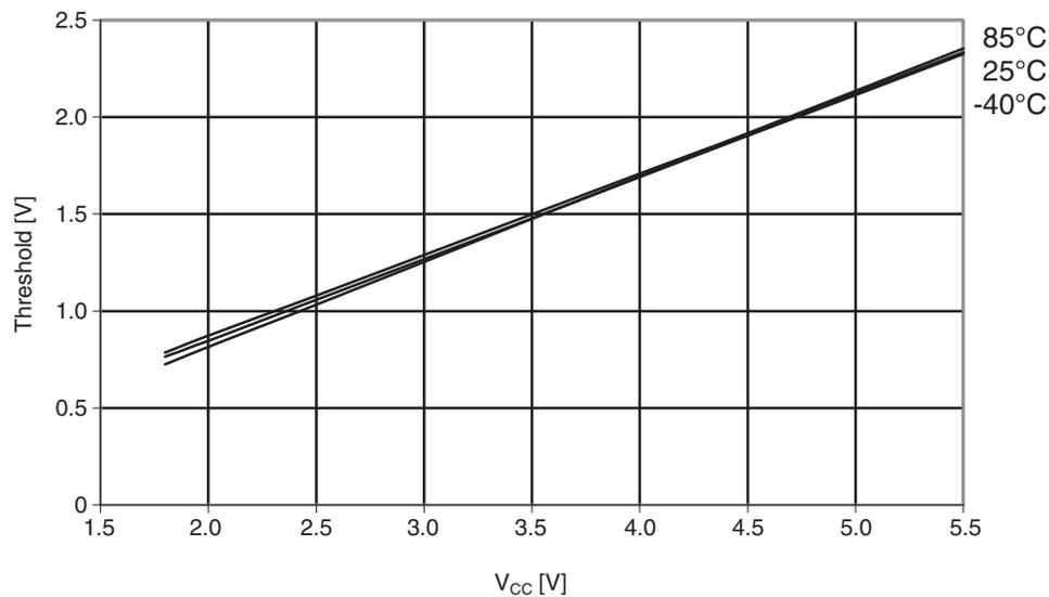
**Figure 30-30. ATmega164A: Reset pin input hysteresis vs.  $V_{CC}$**
