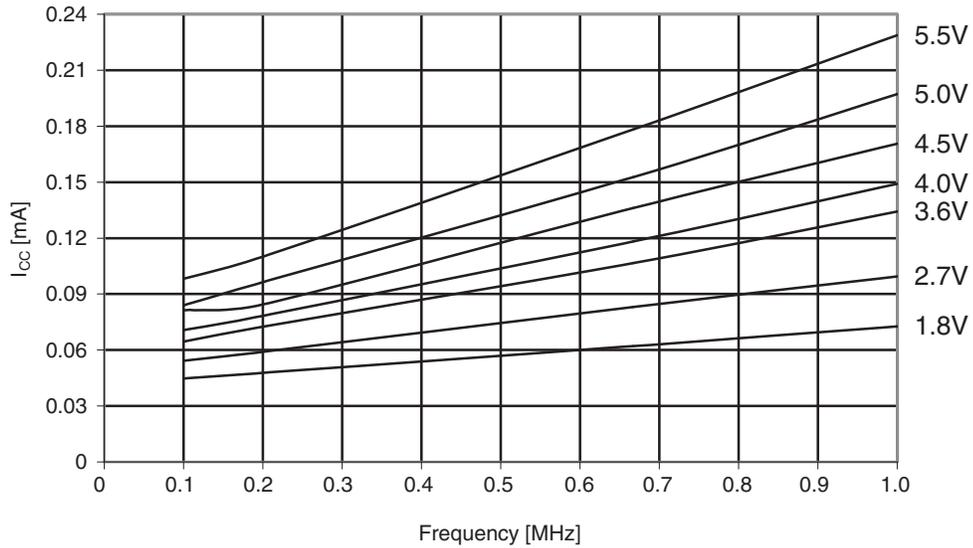
**Figure 30-351. ATmega1284P: Idle supply current vs. frequency (1 - 20MHz)**
