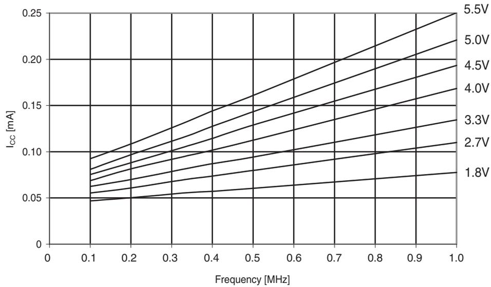
**Figure 30-154. ATmega324PA: Idle supply current vs.  $V_{CC}$  (1 - 20MHz)**
