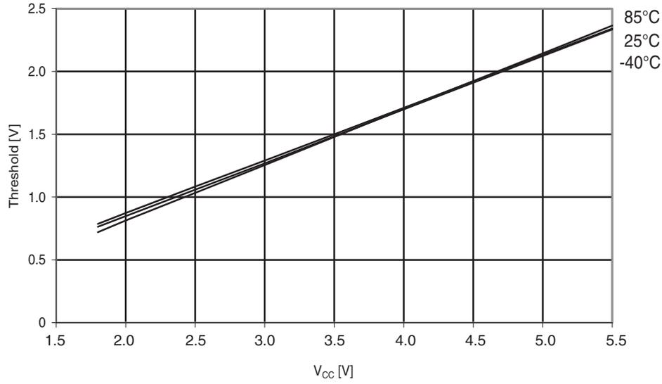
**Figure 30-275. ATmega644PA: Reset pin input hysteresis vs.  $V_{CC}$**
