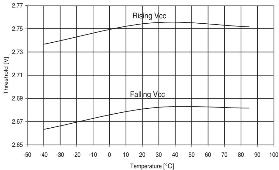
**Figure 30-229. ATmega644A: BOD threshold vs. temperature ( $V_{BOT} = 1.8V$ )**
