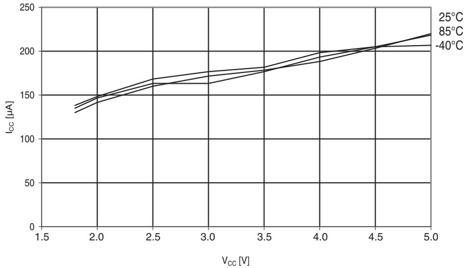
**Figure 30-238. ATmega644A: Analog comparator current vs.  $V_{CC}$**
