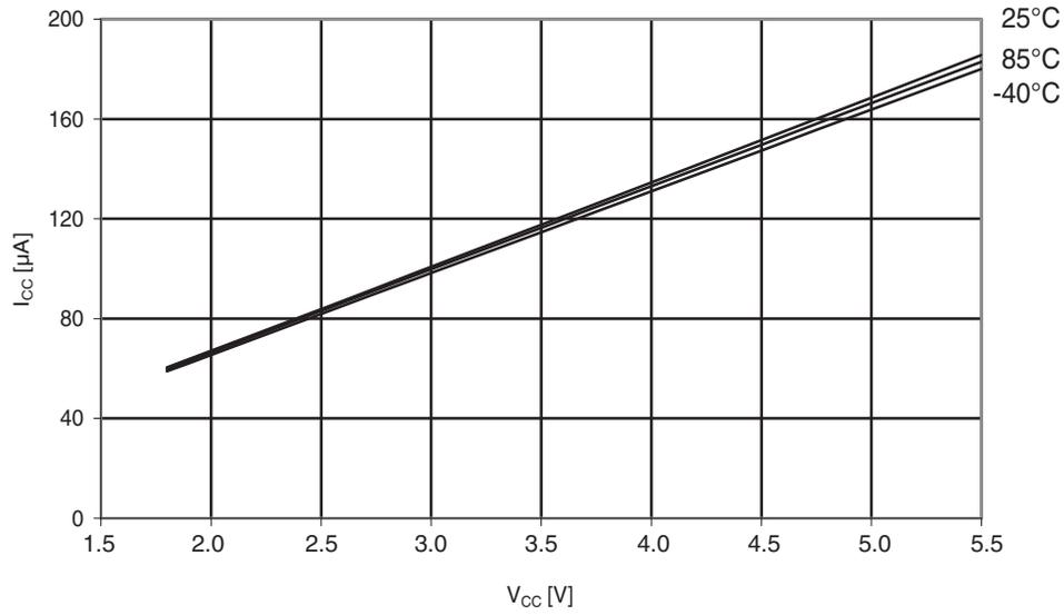
Figure 30-142. ATmega324A: Brownout detector current vs.  $V_{CC}$
