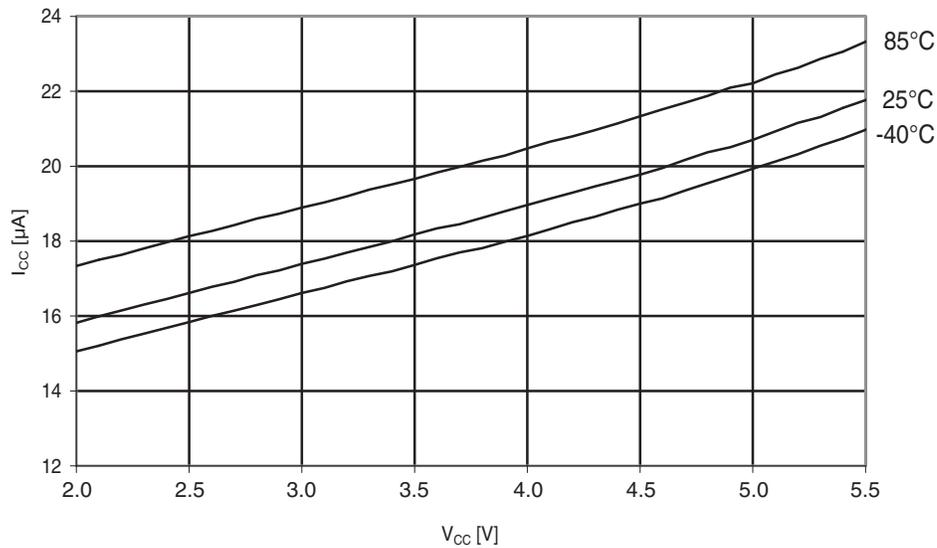
**Figure 30-290. ATmega644PA: Programming current vs.  $V_{CC}$**
