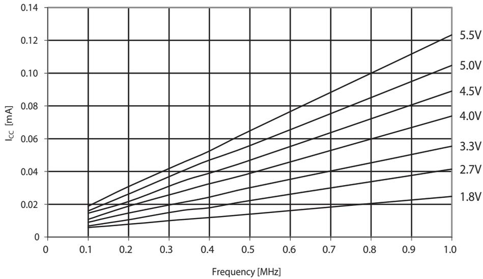
Figure 30-146. ATmega324A: Reset supply current vs. frequency (1 - 20MHz)
