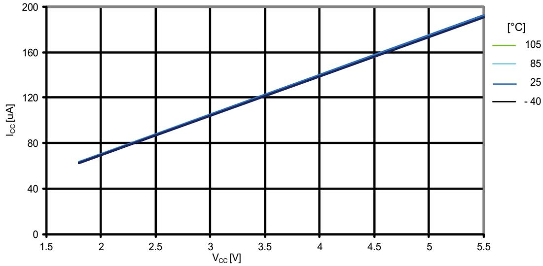
**Figure 31-38. ATmega164PA: Brownout detector current vs.  $V_{CC}$**
