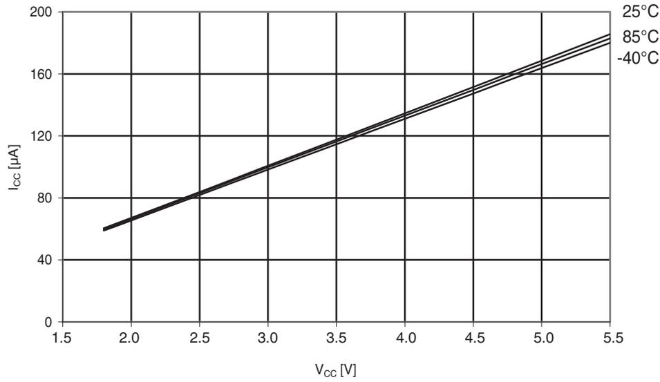
Figure 30-191. ATmega324PA: Brownout detector current vs.  $V_{CC}$
