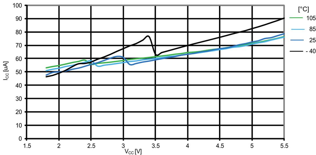
**Figure 31-37. ATmega164PA: AREF external reference current vs.  $V_{CC}$**
