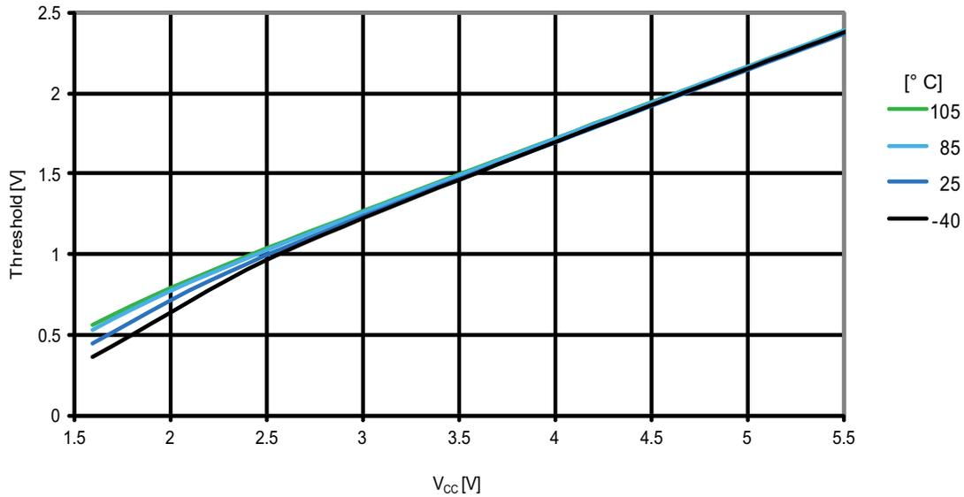
**Figure 31-142. ATmega1284P: I/O pin input hysteresis vs.  $V_{CC}$**
