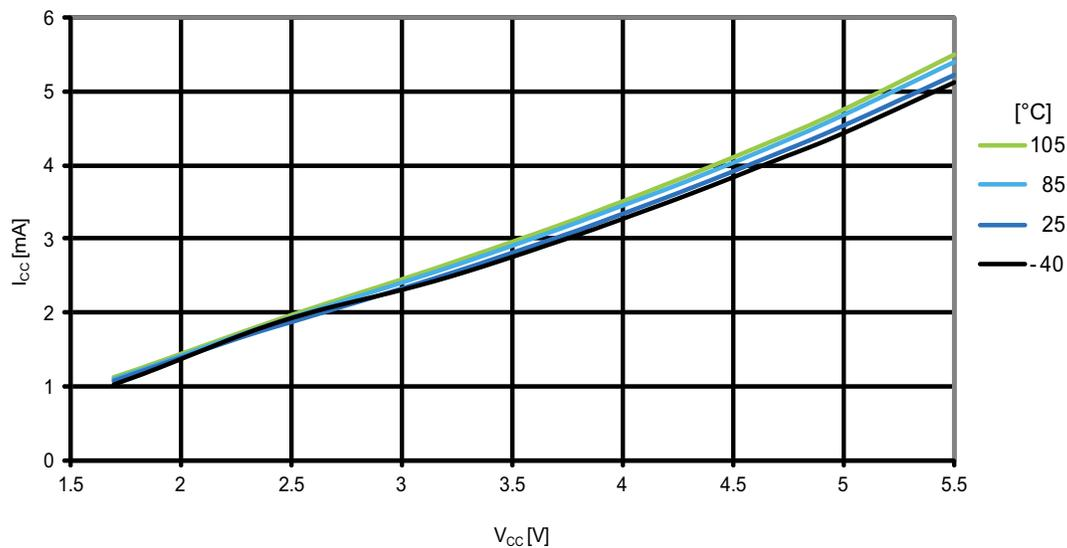
Figure 31-2. ATmega164PA: Active supply current vs. V<sub>CC</sub> (internal RC oscillator, 1MHz)
