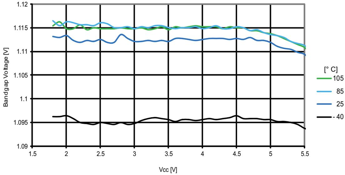
**Figure 31-150. ATmega1284P: Bandgap voltage vs. temperature**
