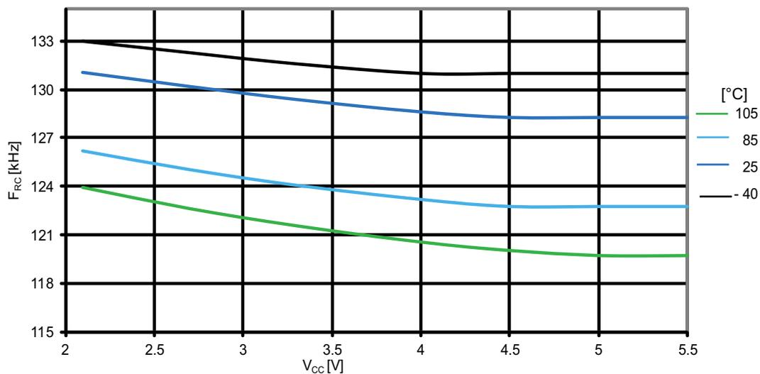
**Figure 31-32. ATmega164PA: Calibrated 8MHz RC oscillator vs.  $V_{CC}$**
