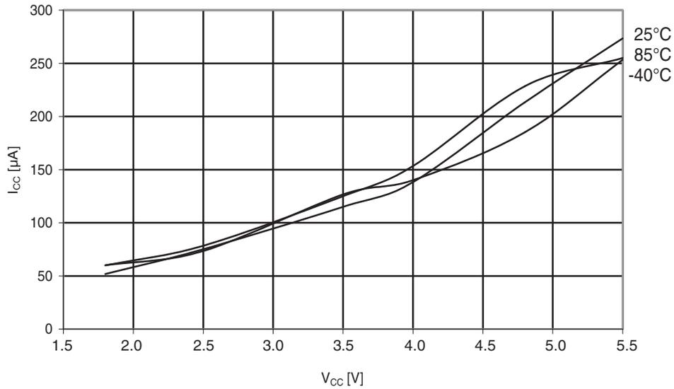
**Figure 30-189. ATmega324PA: Analog comparator current vs.  $V_{CC}$**
