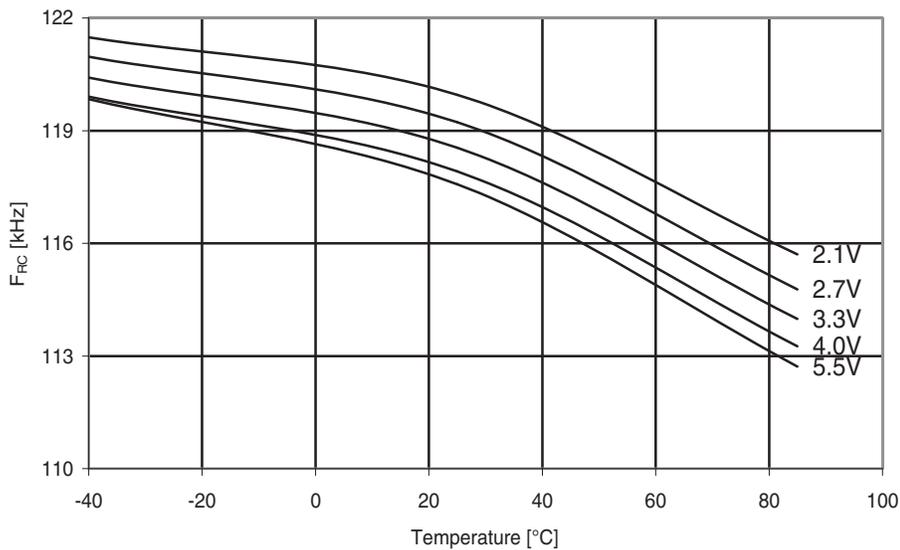
**Figure 30-184. ATmega324PA: Watchdog oscillator frequency vs.  $V_{CC}$**
