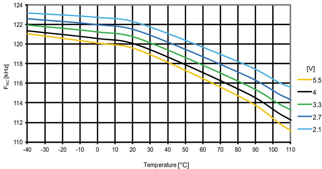
**Figure 31-153. ATmega1284P: Calibrated 8MHz RC oscillator vs.  $V_{CC}$**
