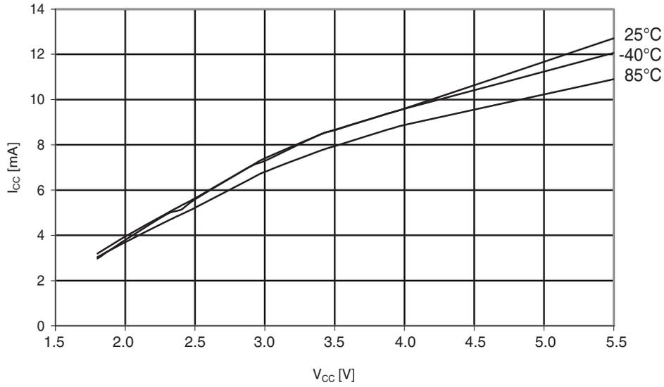
Figure 30-144. ATmega324A: Watchdog timer current vs.  $V_{CC}$
