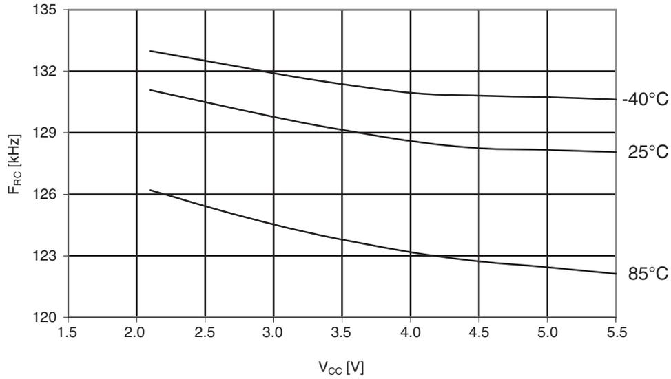
**Figure 30-38. ATmega164A: Calibrated 8MHz RC oscillator vs.  $V_{CC}$**
