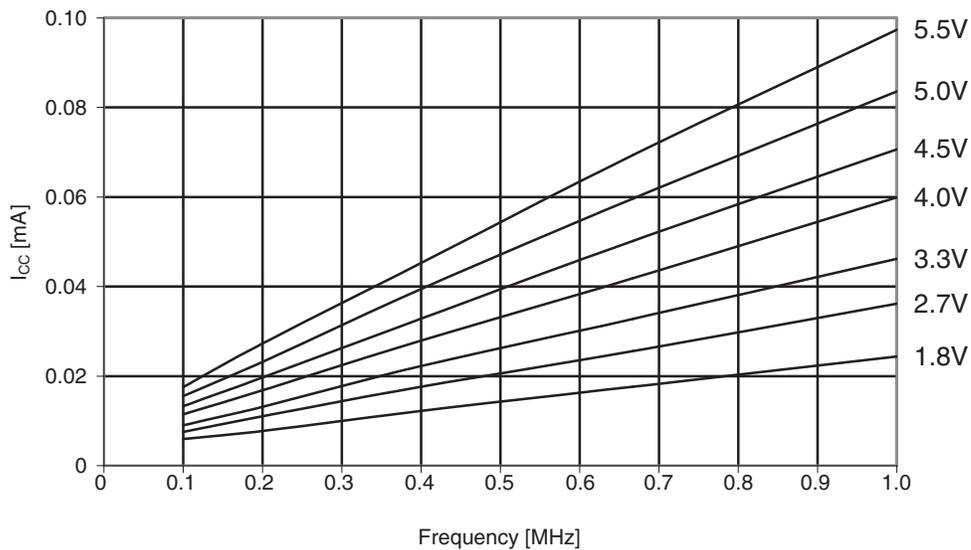
**Figure 30-393. ATmega1284P: Reset supply current vs. frequency (1 - 20MHz)**
