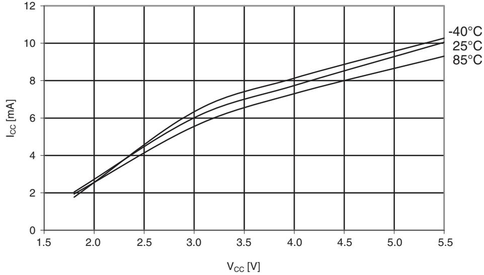
Figure 30-46. ATmega164A: Watchdog timer current vs.  $V_{CC}$
