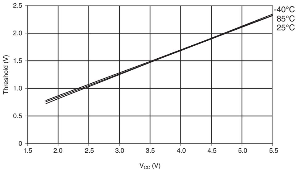
**Figure 30-375. ATmega1284P: Reset pin input hysteresis vs.  $V_{CC}$**
