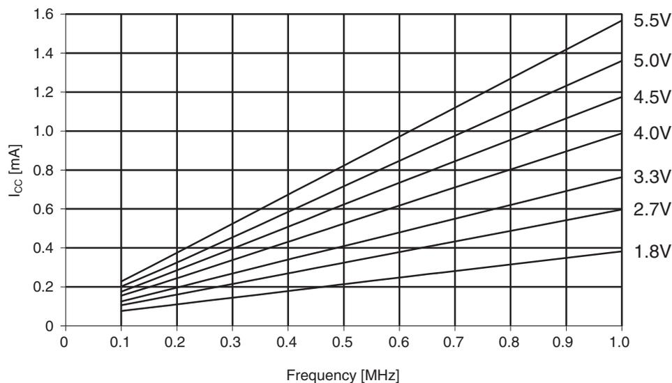
Figure 30-346. ATmega1284P: Active supply current vs. frequency (1 - 20MHz)
