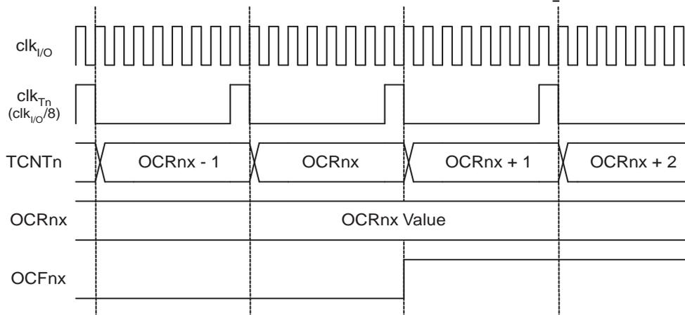
Figure 17-11 on page 156 shows the setting of OCF2A and the clearing of TCNT2 in CTC mode.
