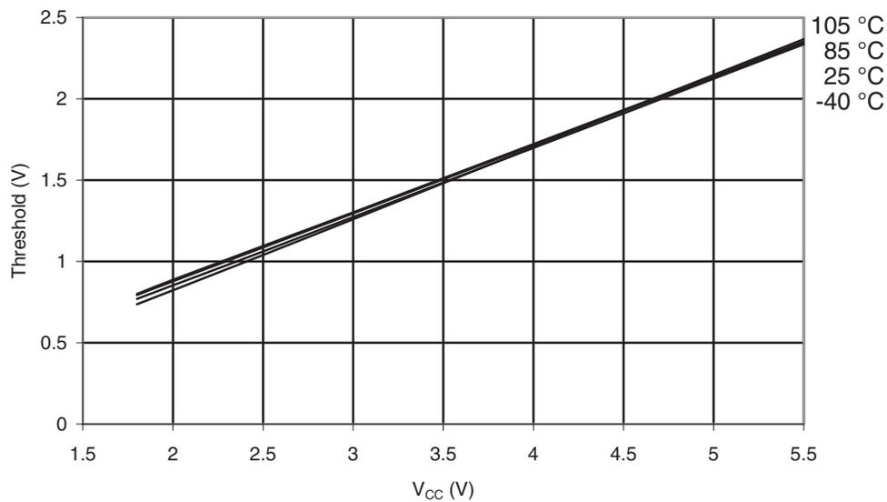
**Figure 31-65. Reset Pin Input Hysteresis vs.  $V_{CC}$**
