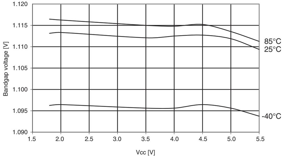
**Figure 30-330. ATmega1284: Bandgap voltage vs. temperature**
