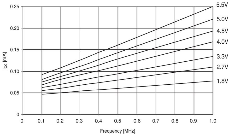
**Figure 30-105. ATmega324A: Idle supply current vs.  $V_{CC}$  (1 - 20MHz)**
