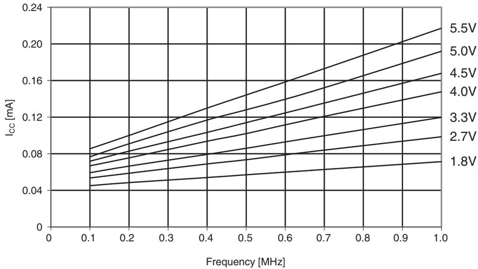
**Figure 30-252. ATmega644PA: Idle supply current vs.  $V_{CC}$  (1 - 20MHz)**
