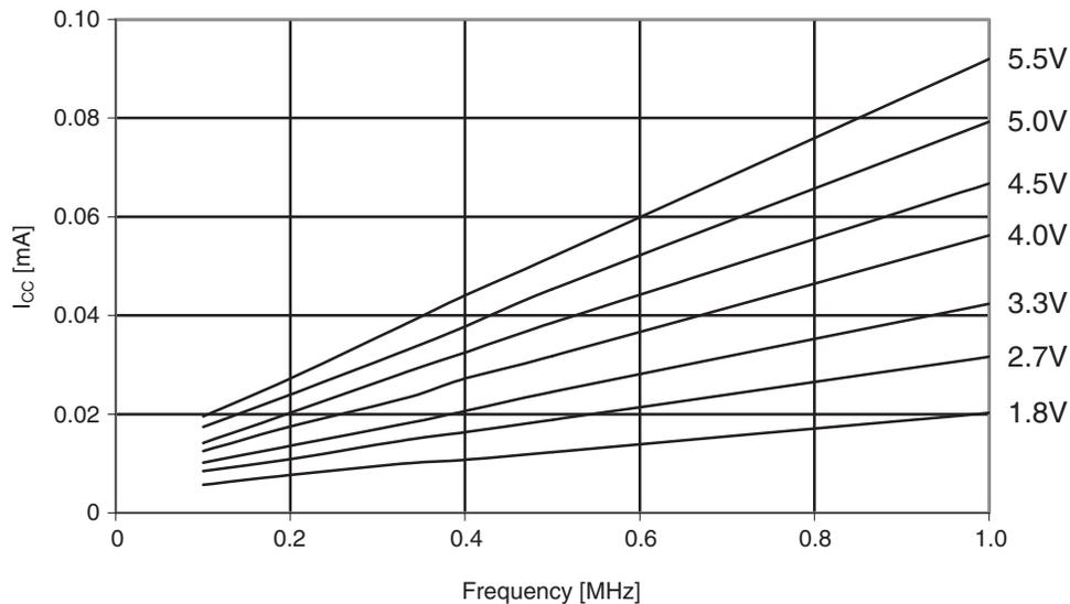
**Figure 30-97. ATmega164PA: Reset supply current vs. frequency (1 - 20MHz)**
