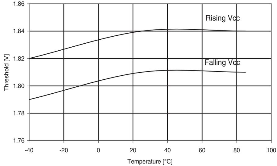
**Figure 30-181. ATmega324PA: Calibrated bandgap voltage vs.  $V_{CC}$**
