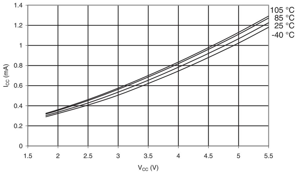
**Figure 31-85. Idle Supply Current vs.  $V_{CC}$  (Internal RC Oscillator, 1 MHz)**
