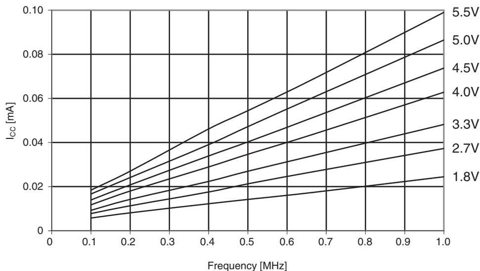
**Figure 30-293. ATmega644PA: Reset supply current vs. frequency (1 - 20MHz)**
