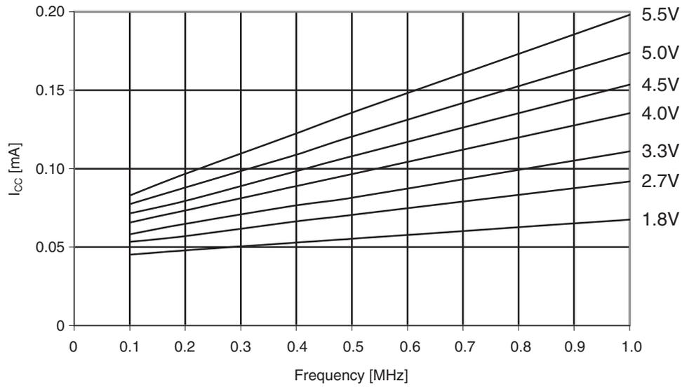
**Figure 30-7. ATmega164A: Idle supply current vs.  $V_{CC}$  (1 - 20MHz)**
