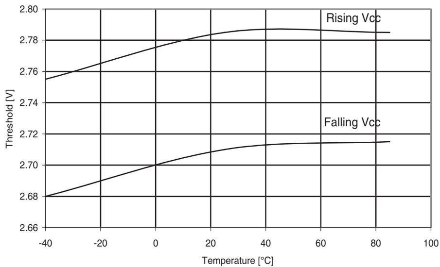
**Figure 30-131. ATmega324A: BOD threshold vs. temperature ( $V_{BOT} = 1.8V$ )**
