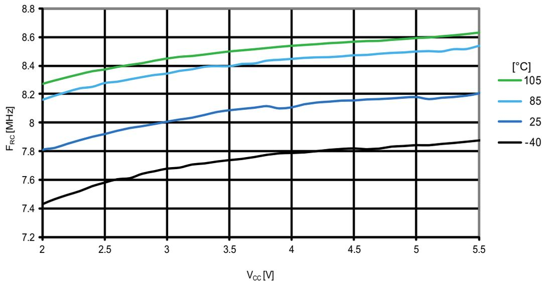
**Figure 31-154. ATmega1284P: Calibrated 8MHz RC oscillator vs. temperature**
