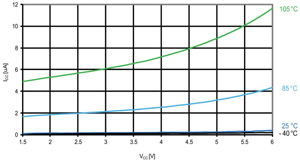
Figure 31-127. ATmega1284P: Power-down supply current vs.  $V_{CC}$  (watchdog timer enabled)
