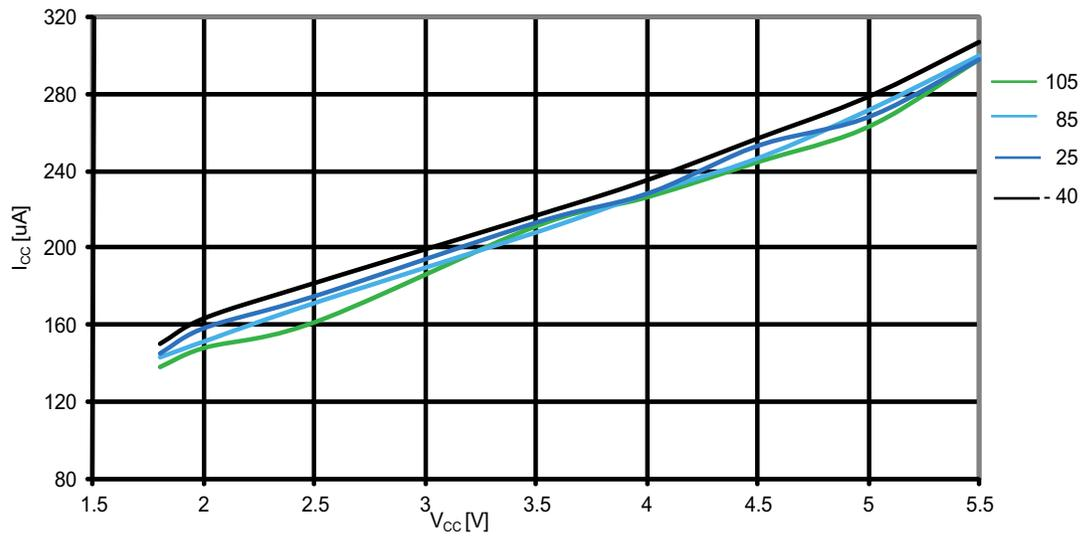
**Figure 31-36. ATmega164PA: Analog comparator current vs.  $V_{CC}$**
