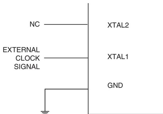
When this clock source is selected, start-up times are determined by the SUT Fuses as shown in [Table 9-15](#).
