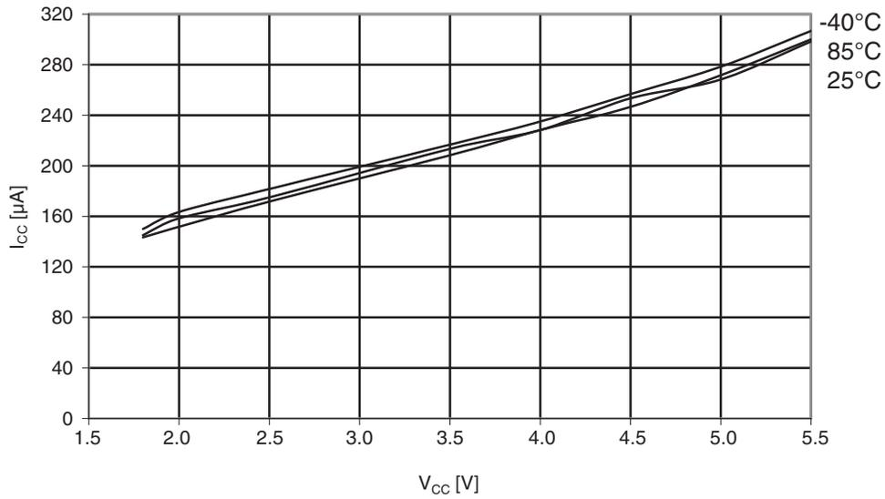
**Figure 30-91. ATmega164PA: Analog comparator current vs.  $V_{CC}$**
