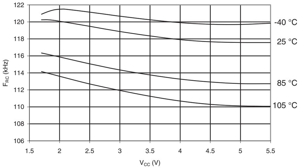
**Figure 31-71. Calibrated 8 MHz RC Oscillator vs.  $V_{CC}$**
