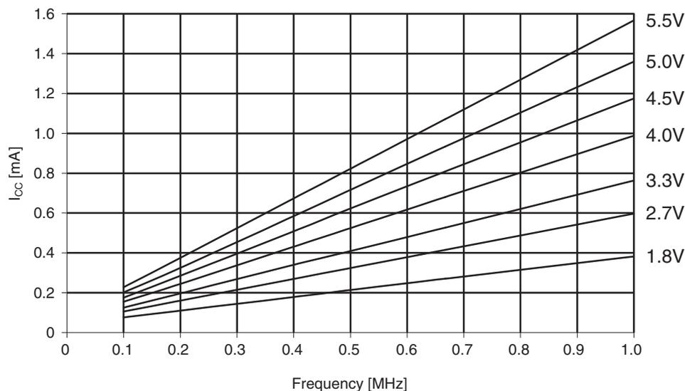
Figure 30-296. ATmega1284: Active supply current vs. frequency (1 - 20MHz)
