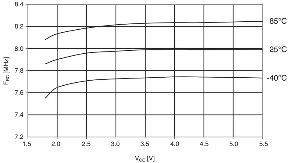
**Figure 30-88. ATmega164PA: Calibrated 8MHz RC oscillator vs. temperature**
