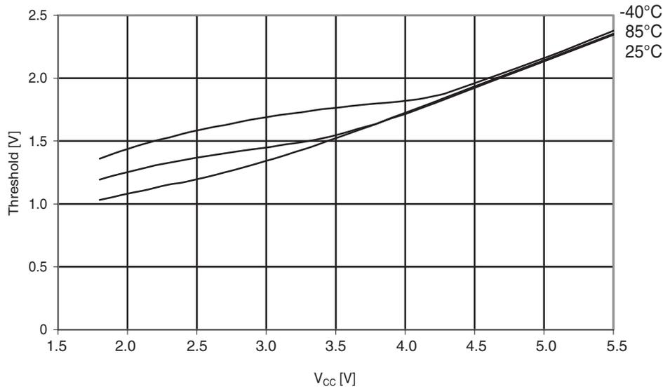
**Figure 30-176. ATmega324PA: Reset pin input threshold vs.  $V_{CC}$  ( $V_{IL}$ , I/O pin read as '0')**
