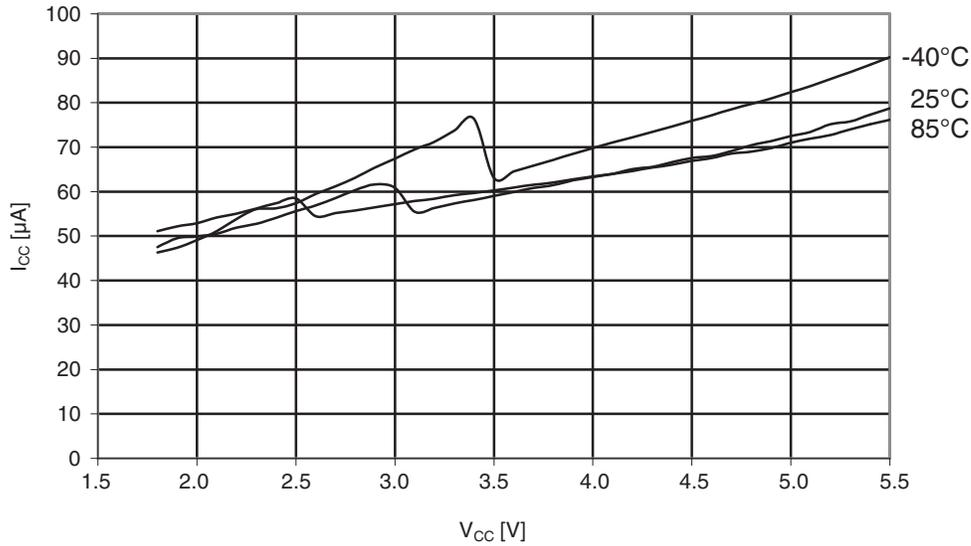
Figure 30-92. ATmega164PA: AREF external reference current vs.  $V_{CC}$
