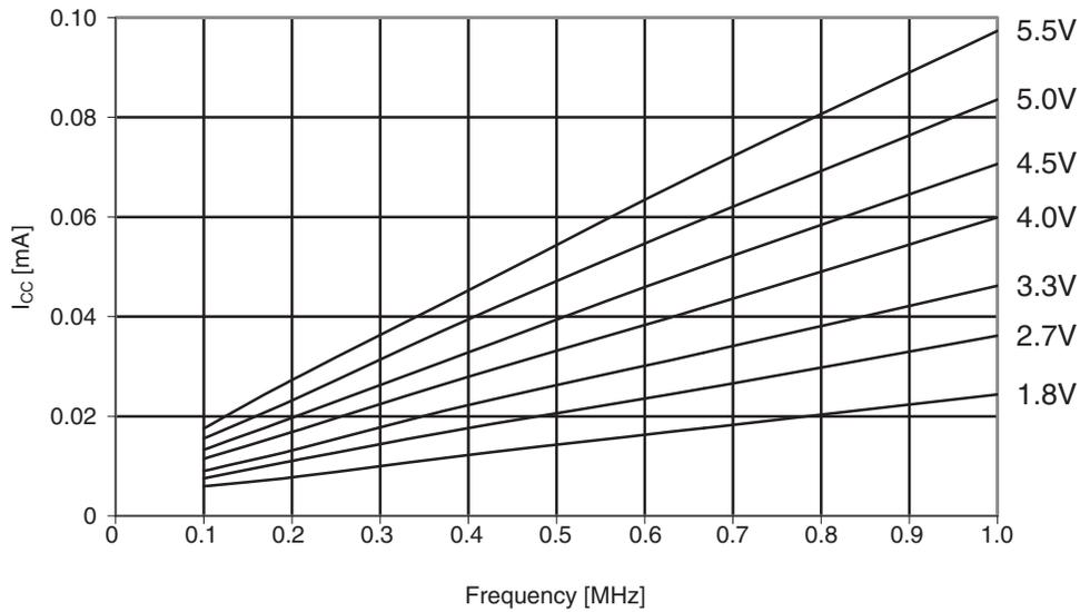
**Figure 30-343. ATmega1284: Reset supply current vs. frequency (1 - 20MHz)**
