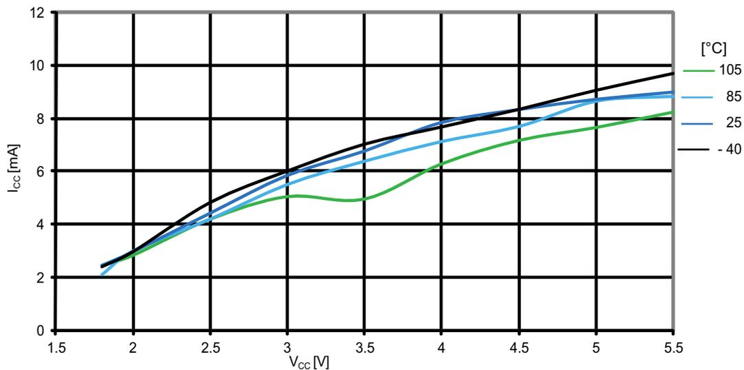
**Figure 31-40. ATmega164PA: Watchdog timer current vs.  $V_{CC}$**
