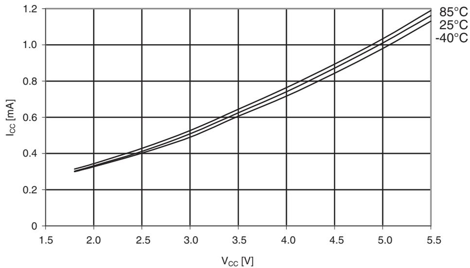
Figure 30-54. ATmega164PA: Active supply current vs.  $V_{CC}$  (internal RC oscillator, 128kHz)
