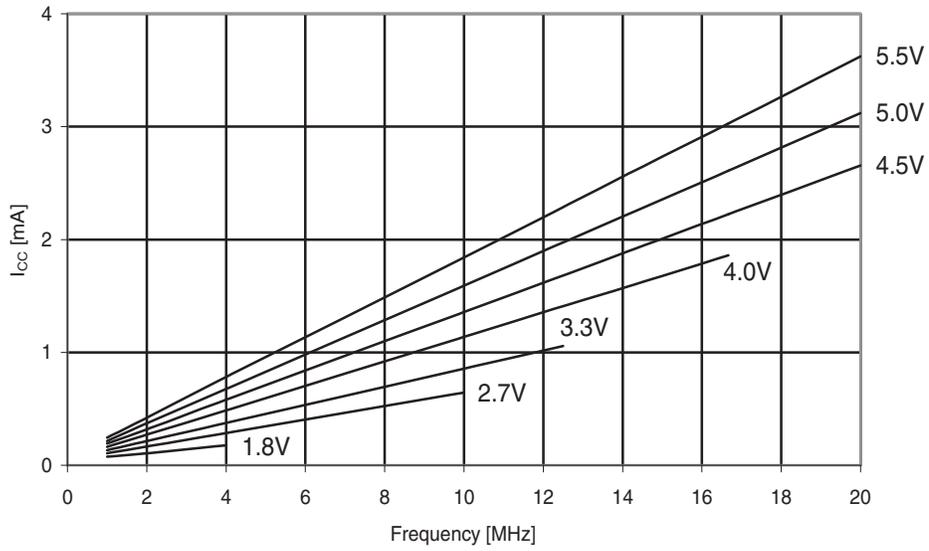
**Figure 30-155. ATmega324PA: Idle supply current vs.  $V_{CC}$  (internal RC oscillator, 8MHz)**
