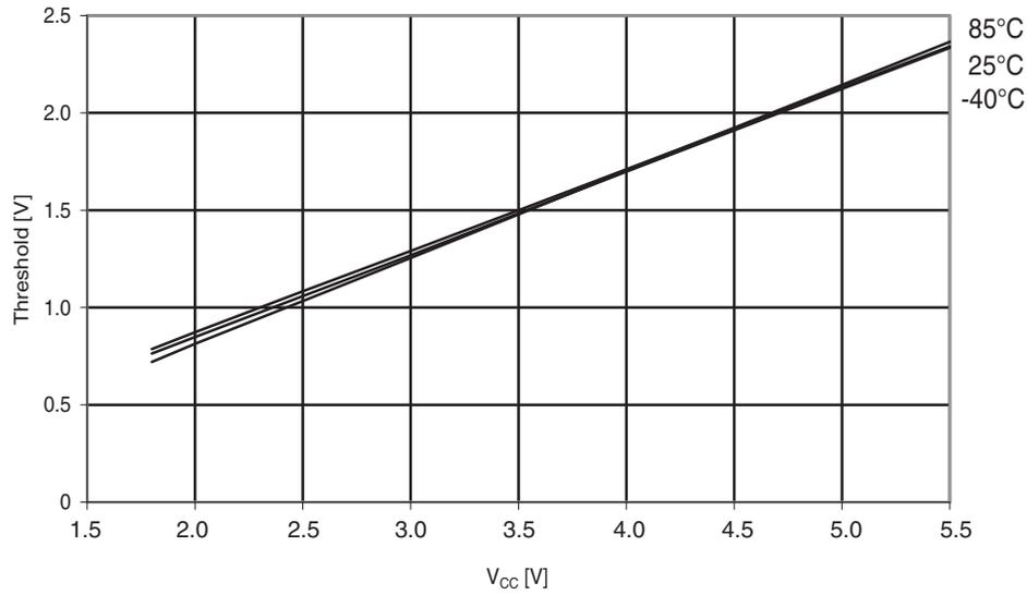
Figure 30-226. ATmega644A: Reset pin input hysteresis vs.  $V_{CC}$
