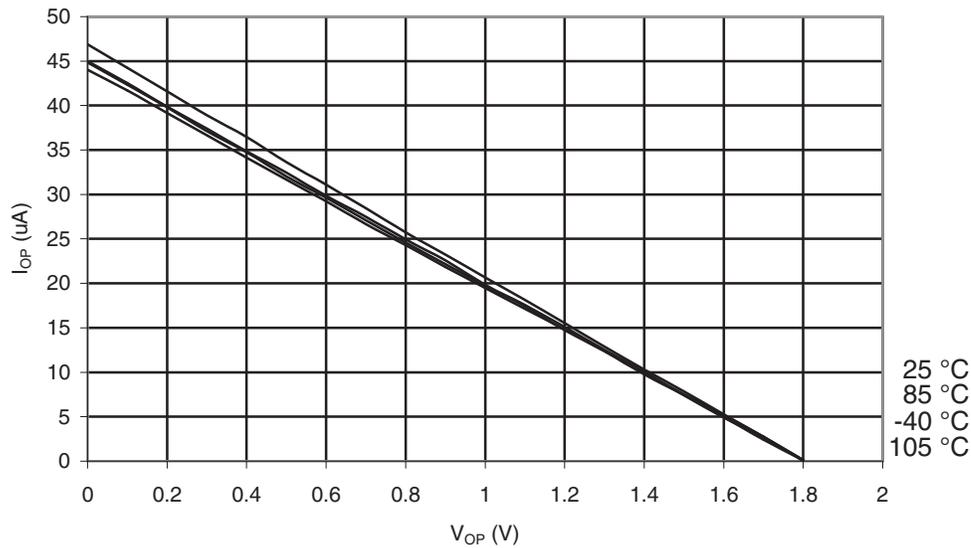
Figure 31-51. I/O Pin Pull-up Resistor Current vs. Input Voltage ( $V_{CC} = 2.7V$ )
