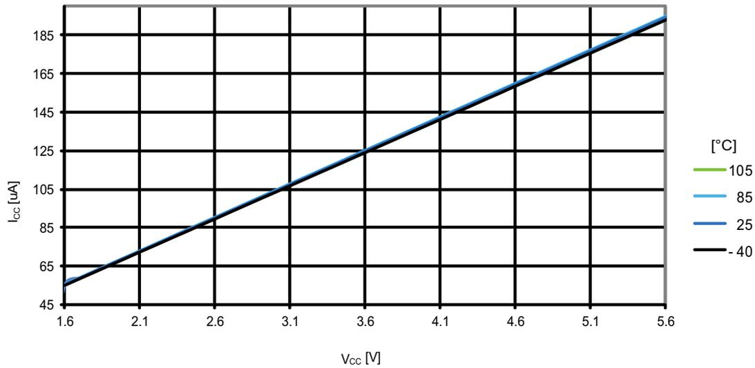
**Figure 31-159. ATmega1284P: Brownout detector current vs.  $V_{CC}$**
