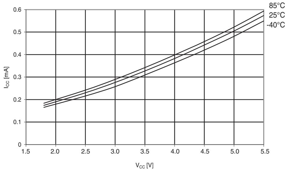
**Figure 30-157. ATmega324PA: Idle supply current vs.  $V_{CC}$  (internal RC oscillator, 128kHz)**
