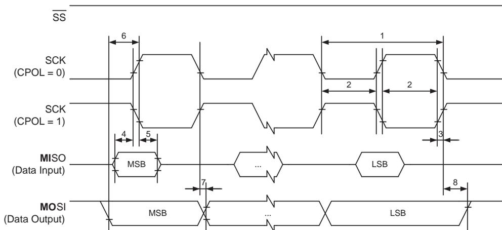
**Figure 28-4. SPI interface timing requirements (Slave mode)**
