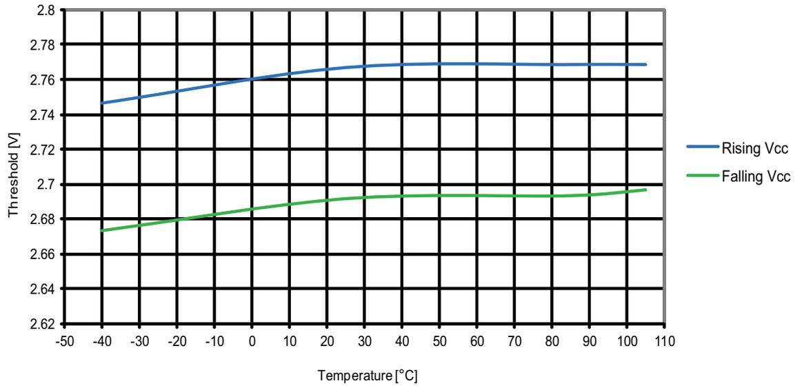
**Figure 31-148. ATmega1284P: BOD threshold vs. temperature ( $V_{BOT} = 1.8V$ )**
