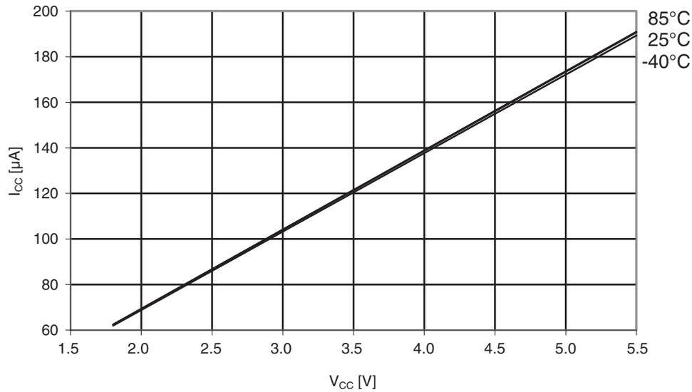
**Figure 30-339. ATmega1284: Brownout detector current vs.  $V_{CC}$**
