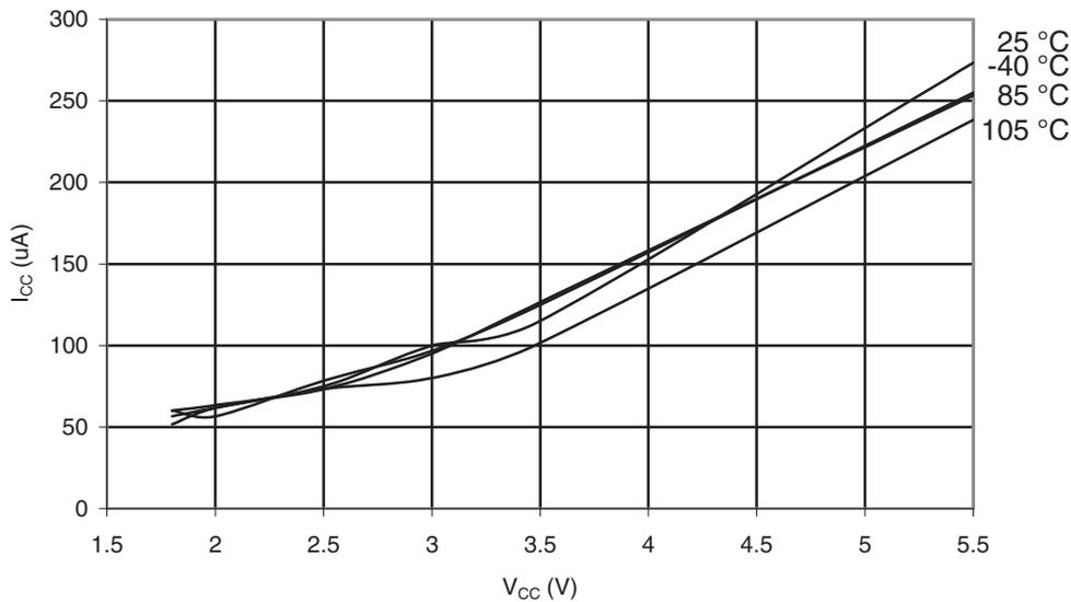
**Figure 31-75. Analog Comparator Current vs.  $V_{CC}$**
