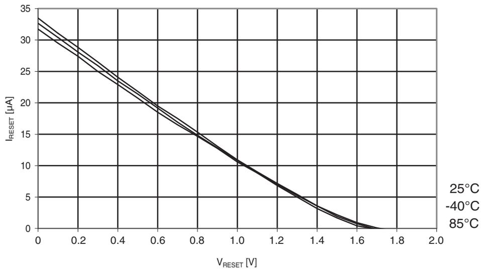
**Figure 30-215. ATmega644A: Reset pull-up resistor current vs. reset pin voltage ( $V_{CC} = 2.7V$ )**
