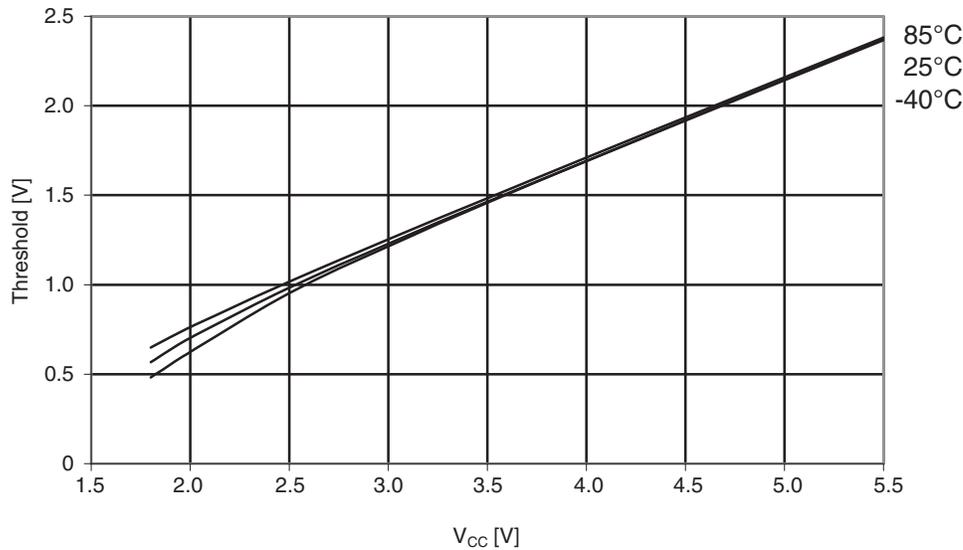
**Figure 30-27. ATmega164A: I/O pin input hysteresis vs.  $V_{CC}$**
