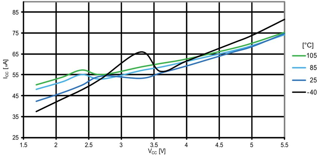
**Figure 31-158. ATmega1284P: AREF external reference current vs.  $V_{CC}$**
