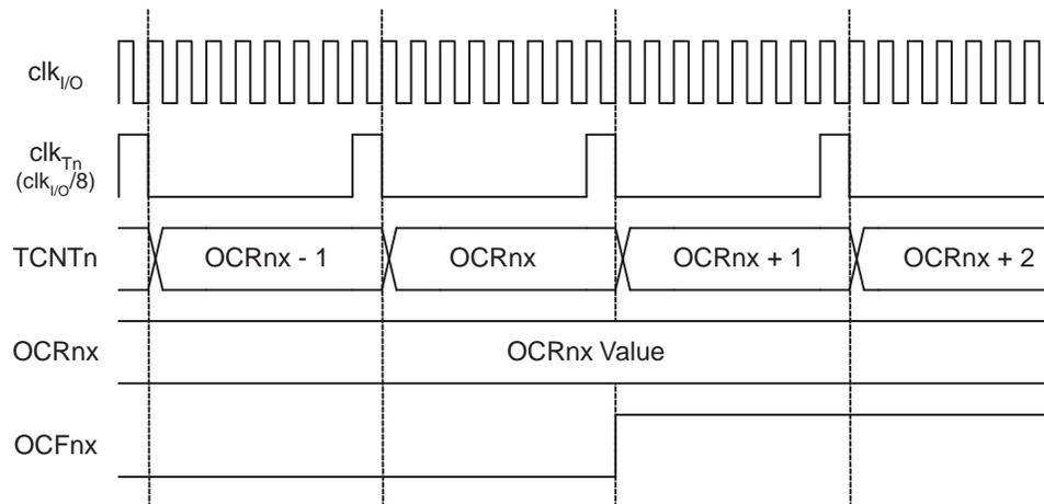
[Figure 16-12](#) shows the count sequence close to TOP in various modes. When using phase and frequency correct PWM mode the OCRnx Register is updated at BOTTOM. The timing diagrams will be the same, but TOP should be replaced by BOTTOM, TOP-1 by BOTTOM+1 and so on. The same renaming applies for modes that set the TOVn Flag at BOTTOM.
