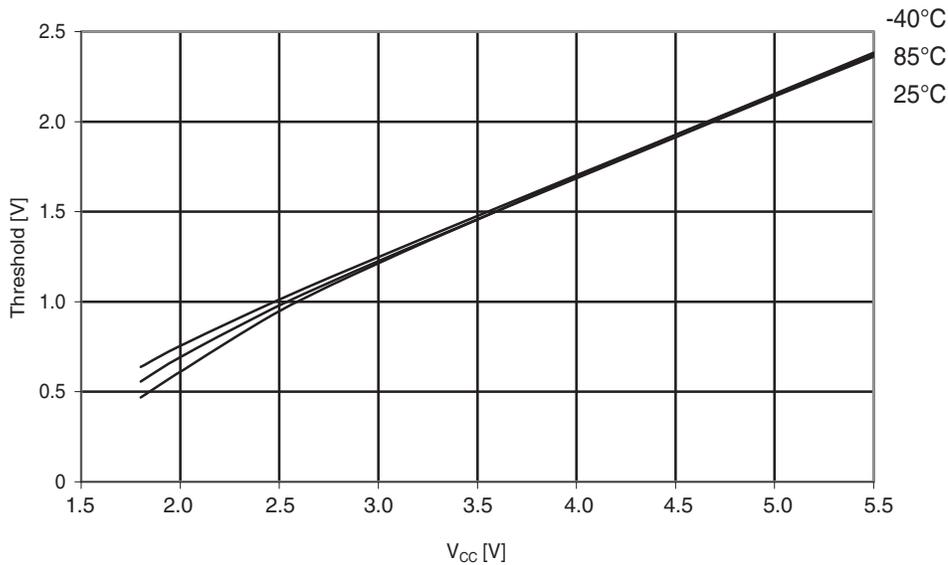
**Figure 30-125. ATmega324A: I/O pin input hysteresis vs.  $V_{CC}$**
