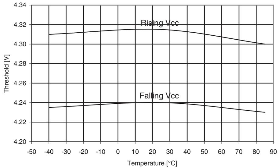
**Figure 30-81. ATmega164PA: BOD threshold vs. temperature ( $V_{BOT} = 2.7V$ )**
