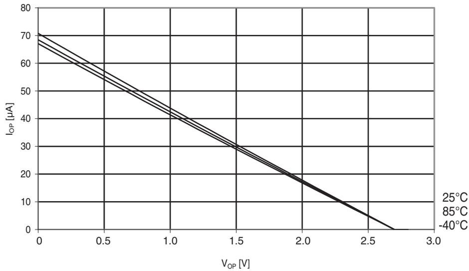
Figure 30-213. ATmega644A: I/O pin pull-up resistor current vs. input voltage ( $V_{CC} = 5V$ )
