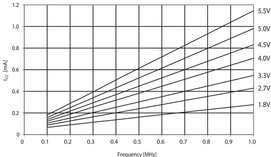
Figure 30-149. ATmega324PA: Active supply current vs. frequency (1 - 20MHz)
