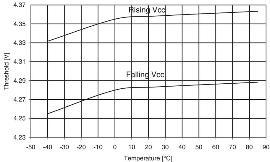
Figure 30-327. ATmega1284: BOD threshold vs. temperature ( $V_{BOT} = 2.7V$ )
