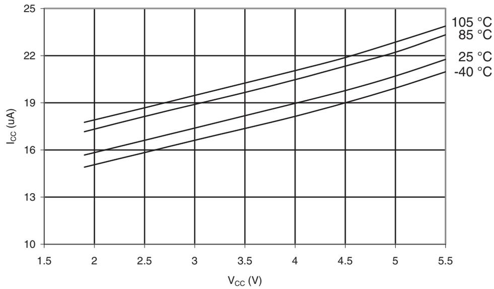
**Figure 31-117. Programming Current vs.  $V_{CC}$**
