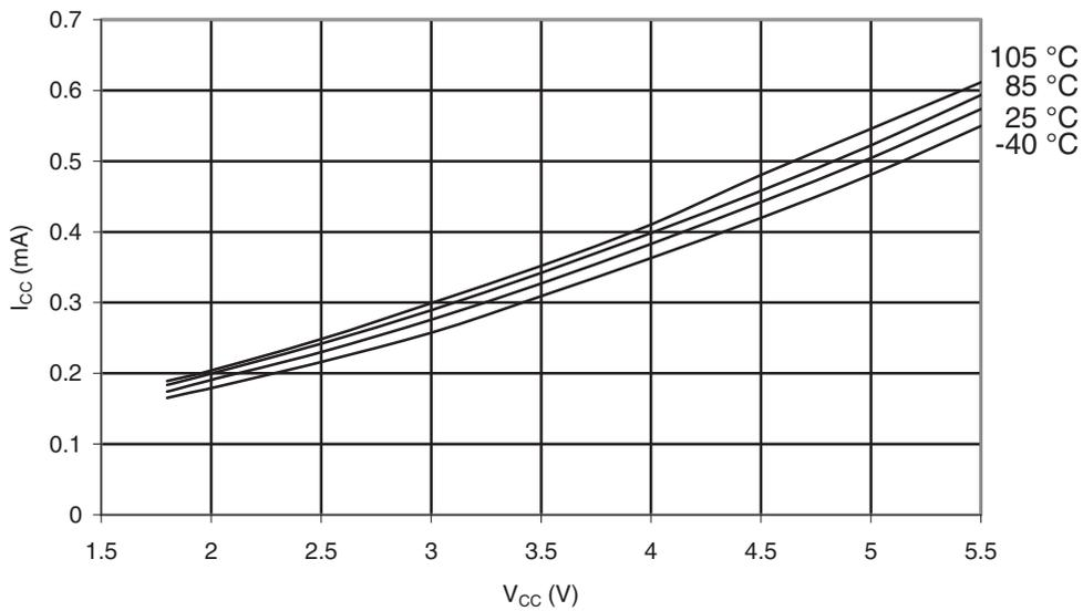
**Figure 31-47. Idle Supply Current vs.  $V_{CC}$  (Internal RC Oscillator, 128 kHz)**
