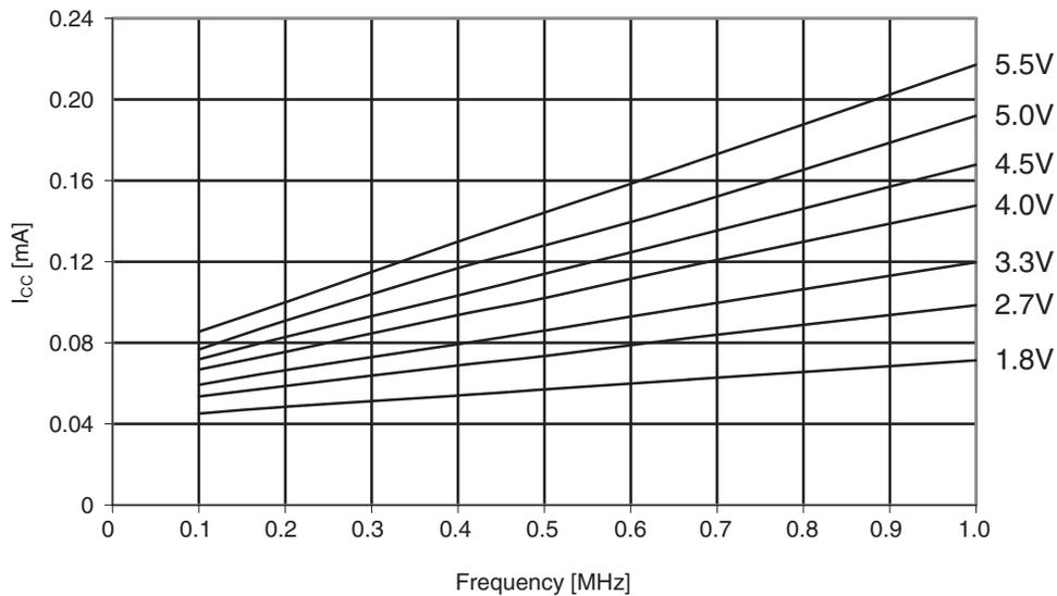
Figure 30-203. ATmega644A: Idle supply current vs.  $V_{CC}$  (1 - 20MHz)
