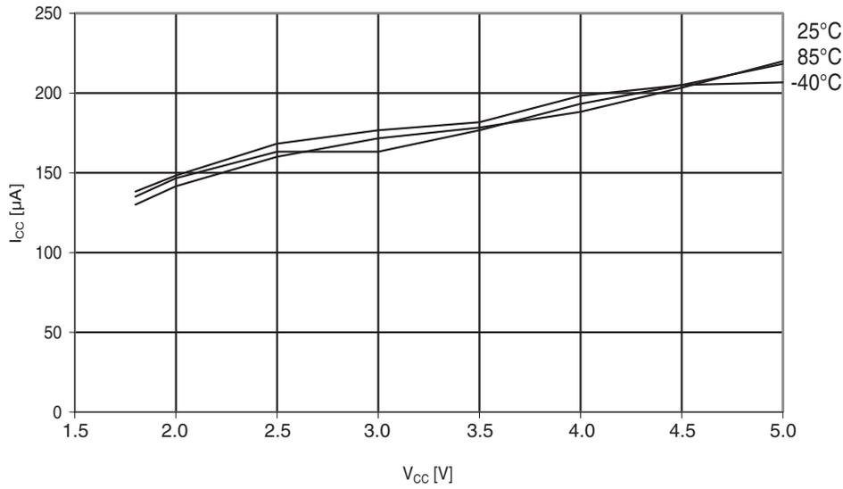
**Figure 30-287. ATmega644PA: Analog comparator current vs.  $V_{CC}$**
