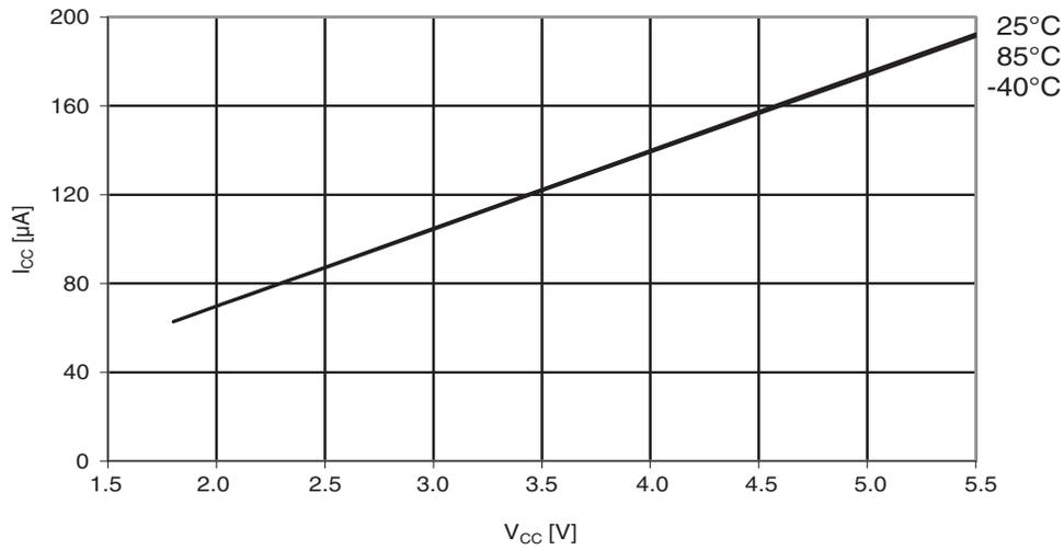
Figure 30-93. ATmega164PA: Brownout detector current vs.  $V_{CC}$
