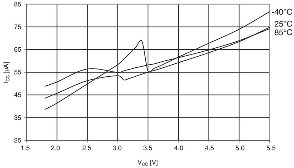
Figure 30-388. ATmega1284P: AREF external reference current vs.  $V_{CC}$
