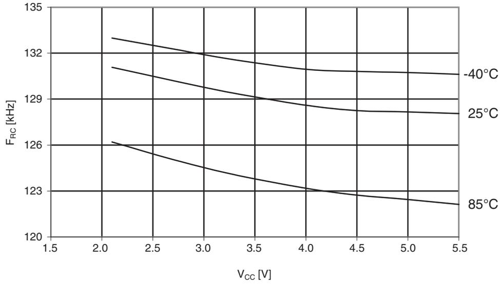
**Figure 30-87. ATmega164PA: Calibrated 8MHz RC oscillator vs.  $V_{CC}$**
