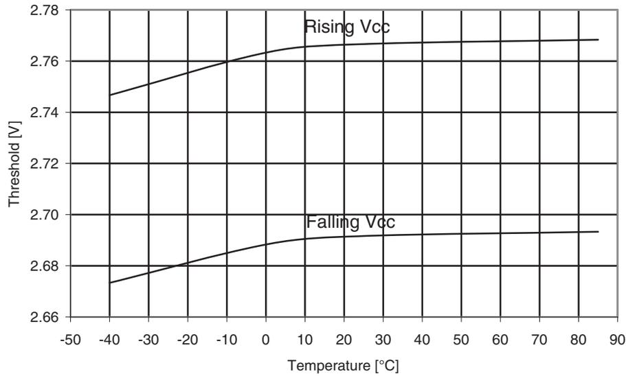
Figure 30-328. ATmega1284: BOD threshold vs. temperature ( $V_{BOT} = 1.8V$ )
