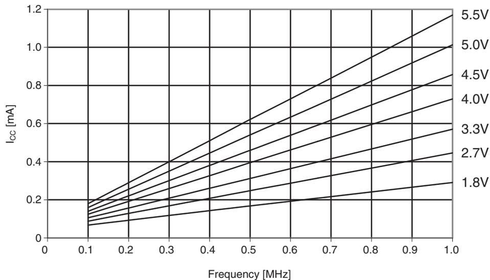
Figure 30-247. ATmega644PA: Active supply current vs. frequency (1 - 20MHz)
