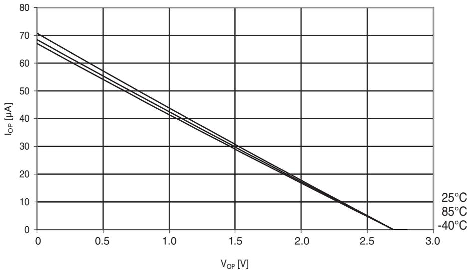
Figure 30-262. ATmega644PA: I/O pin pull-up resistor current vs. input voltage ( $V_{CC} = 5V$ )
