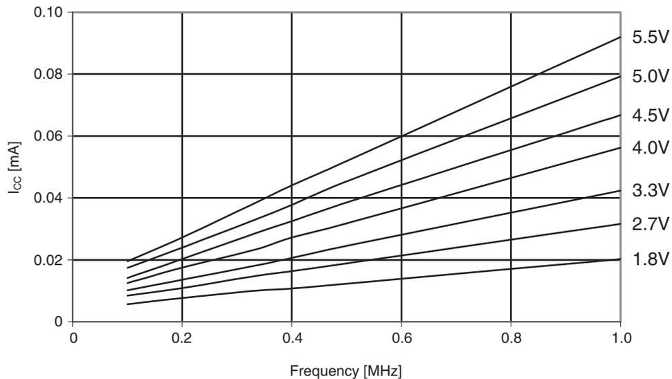
**Figure 30-48. ATmega164A: Reset supply current vs. frequency (1 - 20MHz)**
