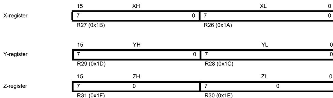
In the different addressing modes these address registers have functions as fixed displacement, automatic increment, and automatic decrement (see the AVR Instruction Set Manual for details).
