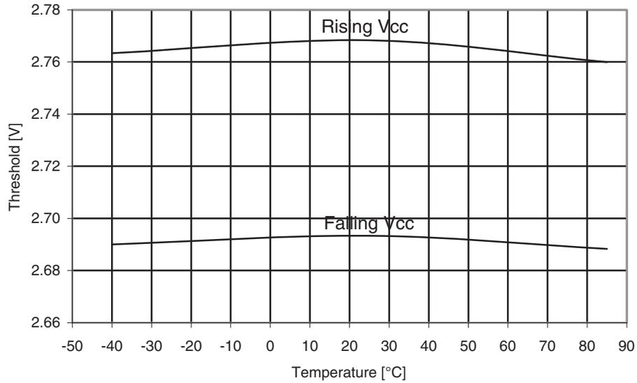
**Figure 30-82. ATmega164PA: BOD threshold vs. temperature ( $V_{BOT} = 1.8V$ )**
