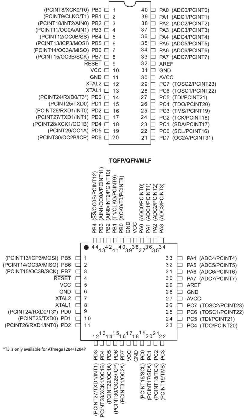
Note: The large center pad underneath the VQFN/QFN/MLF package should be soldered to ground on the board to ensure good mechanical stability.
