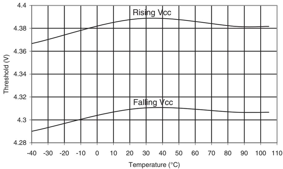
**Figure 31-67. BOD Threshold vs. Temperature ( $V_{CC} = 2.7V$ )**
