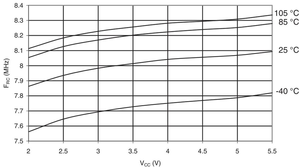
**Figure 31-111. Calibrated 8 MHz RC Oscillator vs. Temperature**
