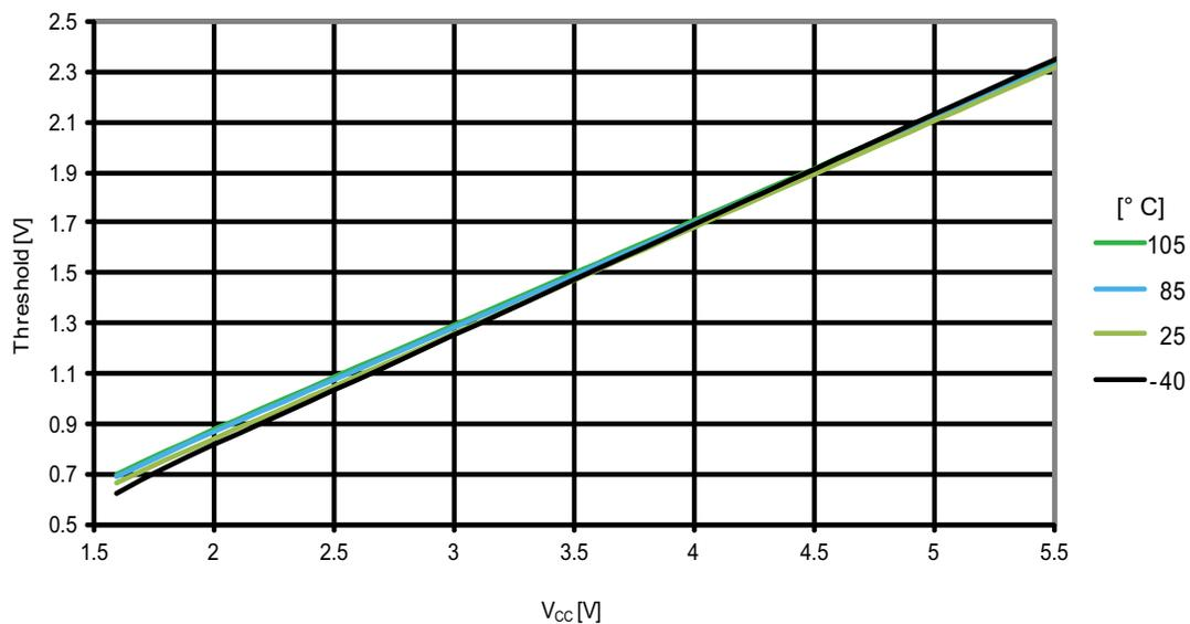
**Figure 31-145. ATmega1284P: Reset pin input hysteresis vs.  $V_{CC}$**
