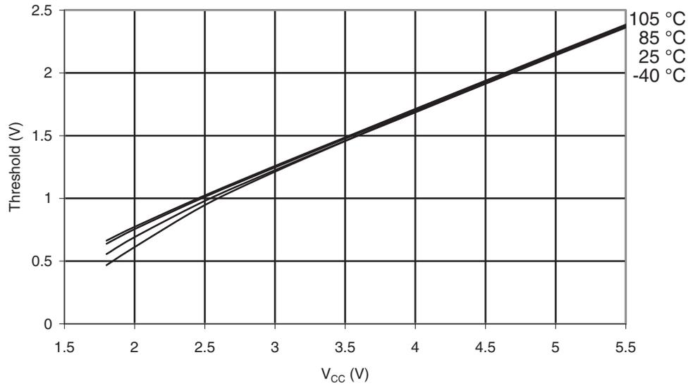
**Figure 31-62. I/O Pin Input Hysteresis vs.  $V_{CC}$**
